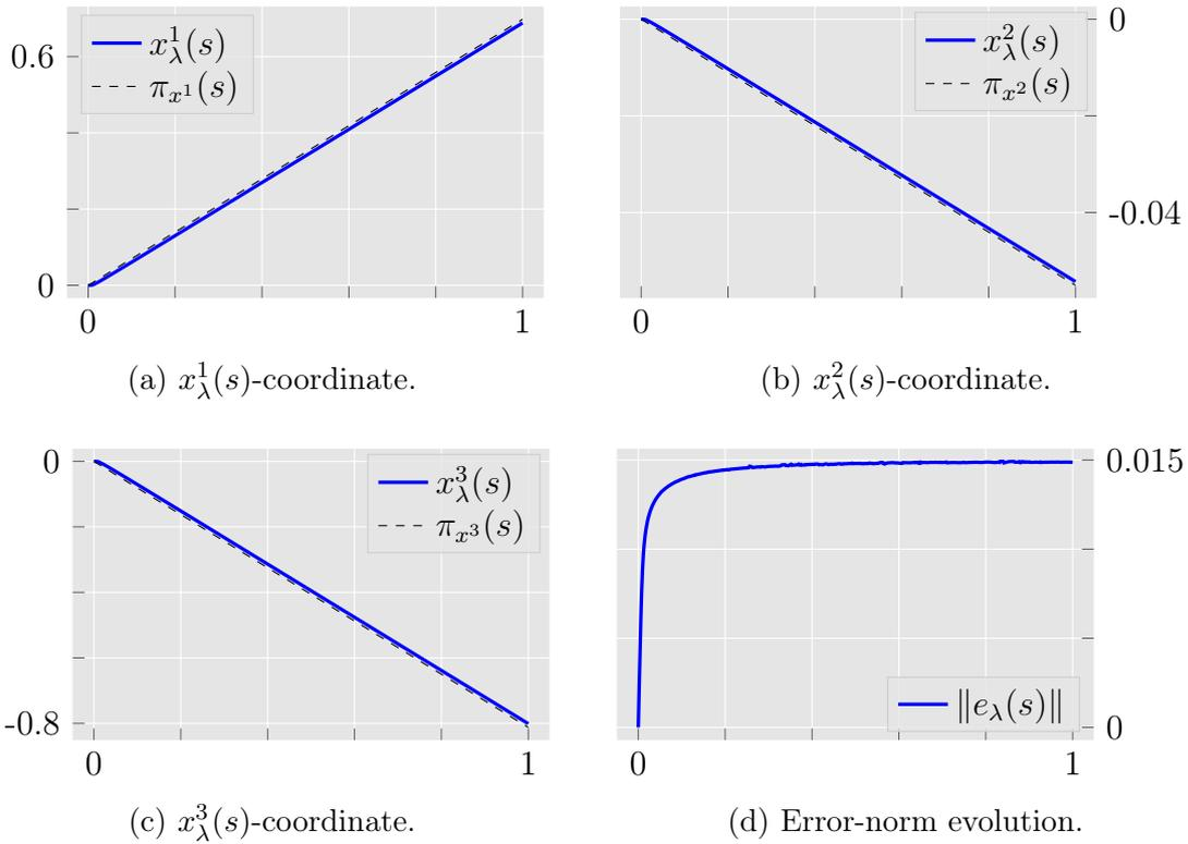
Figure 8.9: Bryant experiment: results of the regularised continuation method for  $\lambda = 10^{-3}$ . Figures 8.9(a) to 8.9(c) show the evolution for  $s \in [0, 1]$  of the coordinate  $x_{\lambda}$  of  $E(\Pi_{\lambda}(s))$ , solid line, and the reference path  $\pi(s)$ , dashed line. Figure 8.9(d) shows the evolution of the error norm  $\|\pi(s) - \pi_{\lambda}(s)\|$  for  $s \in [0, 1]$ .
