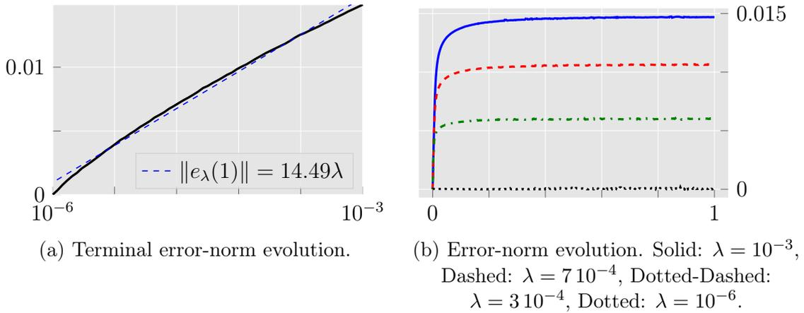
Figure 8.10: Bryant experiment: convergence  $\lambda \rightarrow 0$  of the regularised continuation method. Figure 8.10(a) shows the evolution of the terminal norm error  $\|e_\lambda(1)\|$  against  $\lambda$ , solid line, and the dashed line shows the best linear approximation. Figure 8.10(b) shows the evolution of the norm  $\|e_\lambda(s)\|$ .
