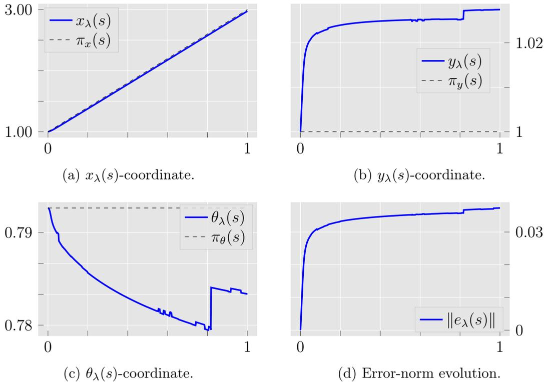
Figure 8.4: Monocycle experiment: results of the regularised continuation method for  $\lambda = 10^{-3}$ . Figures 8.4(a) to 8.4(c) show the evolution for  $s \in [0, 1]$  of the coordinates  $(x_\lambda, y_\lambda, \theta_\lambda)$  of  $E(\Pi_\lambda(s))$ , solid line, and the reference path  $\pi(s)$ , dashed line. Figure 8.4(d) shows the evolution of the error norm  $\|\pi(s) - \pi_\lambda(s)\|$  for  $s \in [0, 1]$ .
