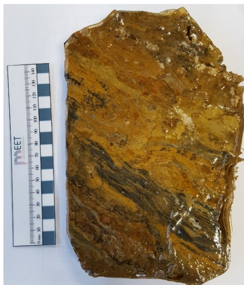
Figure 13: Picture from zone C of a sample from a clay gouge presenting signs of a high amount of dextral shear deformation
