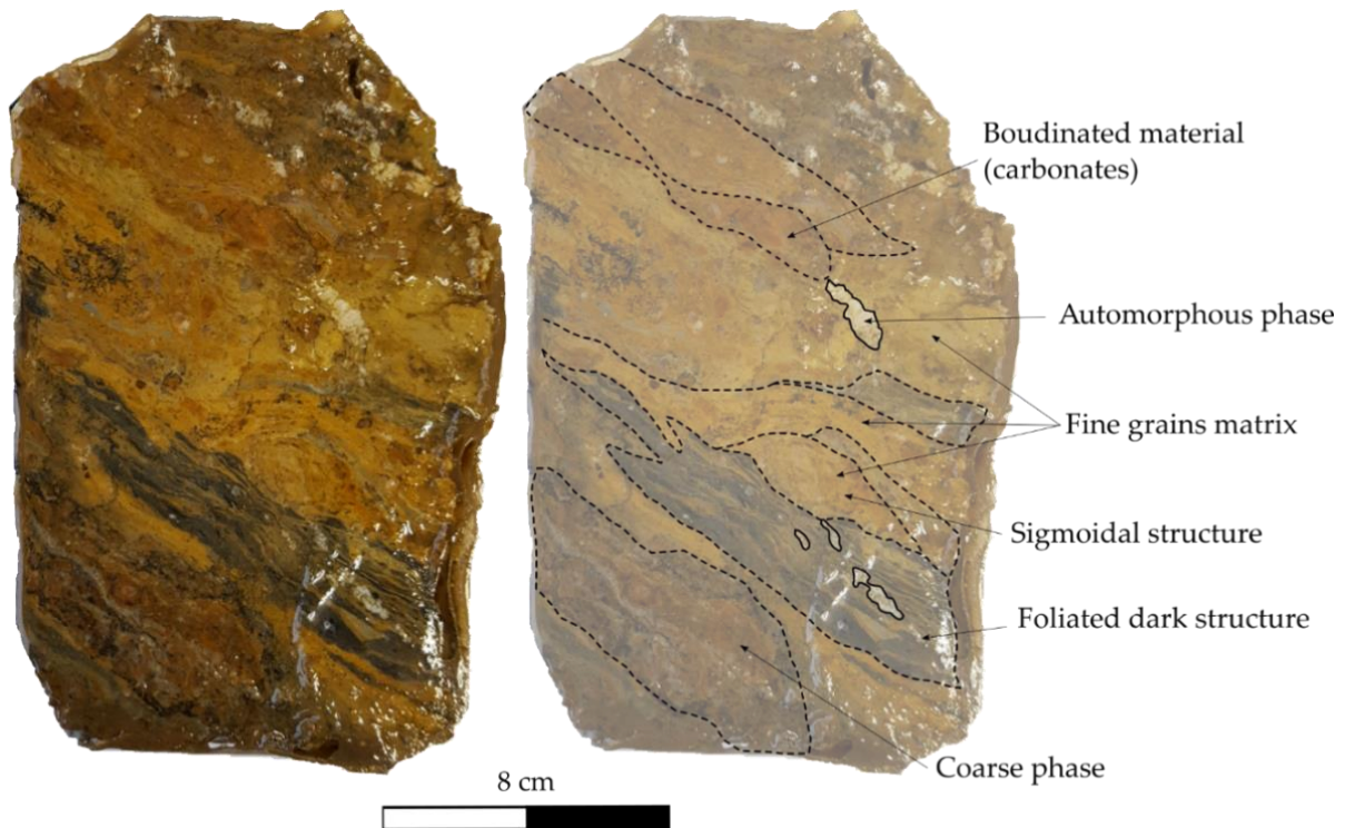
Figure 6-11. Photograph and digitization of sample NH_41 collected from the clay-bearing gouge affected by shear deformation showed by boudinated structures, foliated material and sigmoid.
