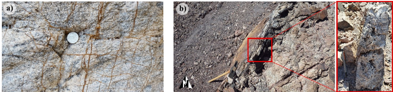
Figure 11: Pictures from zone A presenting a) an altered granite rich in carbonates veins and b) a fracture filled by automorphic barite
