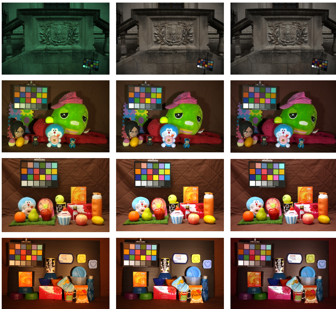
Figure 7.1: Left : input image. Center : output image after white balance using the von Kries CAT. Right : output image after white balance using the normalized Lorentz boost CAT. The white balanced images have been obtained using the same illuminant estimation, performed manually on the white patch of the color checker present in each image. The image of the first row belongs to the ColorChecker Dataset [59, 142], while the others belong to the NUS Indoor Dataset [30].
