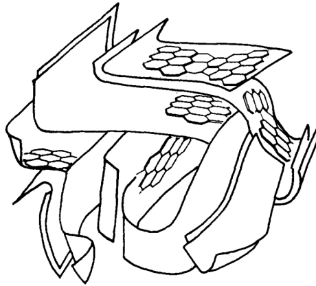
Figure 1.3: Schematic representation of a disordered carbon material highlighting the presence of porosity between the defective and distorted graphene layers [22].
