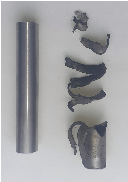
Figure I.3: Fragmentation pattern obtained after the initiation of a physical mixture of carbon C and sodium perchlorate at a density of 1.00 \text{ g/cm}^3 and heavily confined in a 20 mm steel tube (a pristine tube is shown on the left side of the picture).
