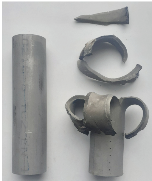
Figure I.1: Fragmentation pattern obtained after the initiation of bare sodium perchlorate at a density of 1.39 \text{g}/\text{cm}^3 and heavily confined in a 30 mm steel tube (a pristine tube is shown on the left side of the picture).
