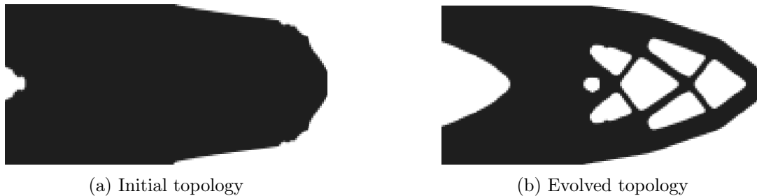
Figure 1.5: Topology optimization (source: Shape Optimization Group at CMAP).
