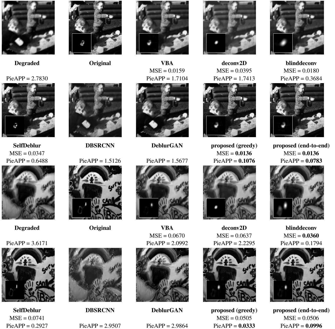
Figure 5.10: Ground-truth image/blur, degraded image, restored images (with PicAPP index) and estimated blurs (with MSE score) when available, for various methods, on two examples in the test set of Dataset 3 .
