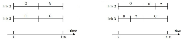
Figure 4.2: The cycle time in the classical model, and in the new model. G: green, R: red, Y: yellow.
