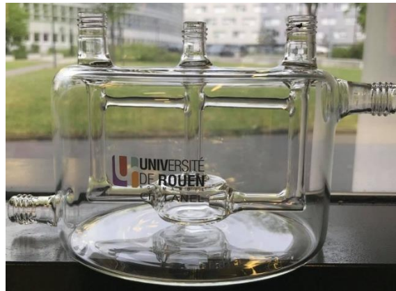
Figure III- 10: Manufactured second prototype of the mixing piece.
