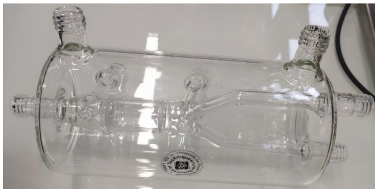
Figure III- 6: Photos of the first prototype of the temperature regulated Y-shaped connection.
