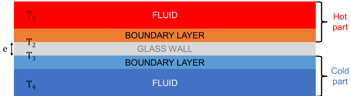
Figure III- 4: Schematic representation of the simplified system for the calculation of H .
