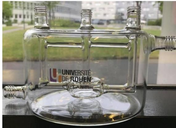
*Figure III- 10: Manufactured second prototype of the mixing piece.*
