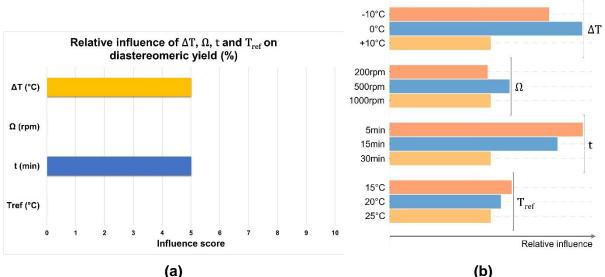
Figure E- 5: Results from Azurad for the diastereomeric yield: (a) Relative influence of the temperature difference  $\Delta T$ , the rotation speed  $\Omega$ , the residence time t and the reference temperature  $T_{ref}$  on the diastereomeric yield. (b) Total effect plot taken from Azurad; for every factor, the bars give the relative effect of each level to improve the diastereomeric yield.
