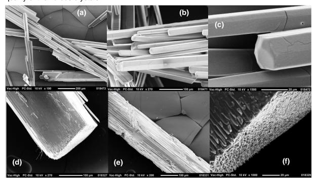
Figure II- 15: (a–c) SEM photographs of pure S-Ibu-S- $\alpha$ MBA. (d–f) SEM photographs of ss-S-Ibu-S- $\alpha$ MBA at the limit of the solid solution (X<sub>R-Ibu-S- $\alpha$ MBA</sub> = 14%).
