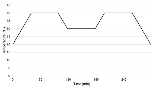
Figure IV- 2: Temperature cycle imposed to the experiment B1 (5 g scale). All rates were of 0.5 °C.min<sup>-1</sup>, and all hold times of 1 h.
