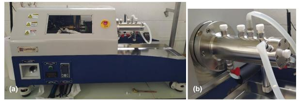
Figure III- 1: Photos of the Couette-Taylor reactor: (a) whole device, (b) closed reactor part.
