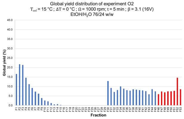
Figure IV- 17: Global yield distribution of experiment O2. The conditions are that of experiment O1, but with a lower supersaturation level  $\beta$  of 3.1. Blockage occurred after fraction 45. It was eliminated by heating up the CT reactor to 40 °C and flushing it with technical ethanol. Fractions 46 to 53 (red) were collected after the return of the crystallizer to the reference temperature of 15 °C.
