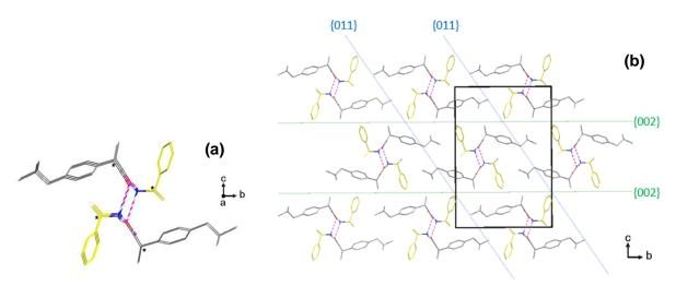
Figure II- 11: Molecular chain of S-Ibu-S-α-MBA spreading along the 'a' axis. The carbon atoms are displayed in yellow for S-αMBA and in grey for S-Ibu. Chiral carbon for both molecules is highlighted with an asterisk. (b) Projection along the 'a' axis of the S-Ibu-S-α-MBA crystal structure. The slices {002} and {011} are shown; their surfaces are clearly hydrophobic.
