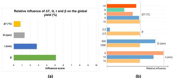
Figure E- 7: Results from Azurad for global yield: (a) Relative influence of the temperature difference  $\Delta T$ , the rotation speed  $\Omega$ , the residence time t and the supersaturation ratio  $\beta$  on the global yield. (b) Total effect plot taken from Azurad; for every factor, the bars give the relative effect of each level to improve global yield.
