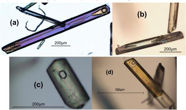
Figure II- 31: Micrographs of particles of pure S-Ibu-S- $\alpha$ MBA obtained by cooling from 40 °C to 20 °C (a-b) in pure ethanol (99.8 %) and (c-d) in azeotropic ethanol (EtOH/H<sub>2</sub>O 95/5 w/w); taken by optical polarized light microscopy.
