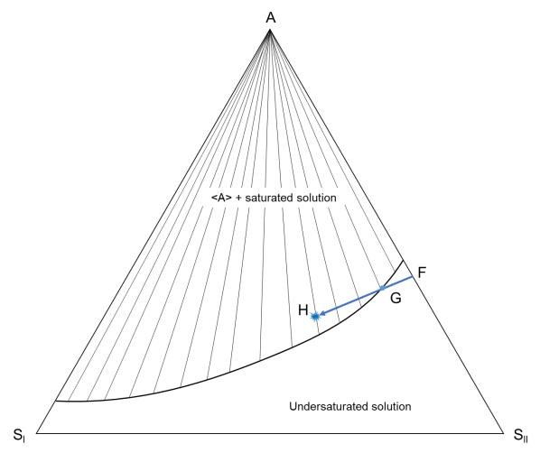
Figure I- 3: Ternary isotherm depicting crystallization by antisolvent addition, with solute A, solvent  $S_1$  (bad solvent or anti-solvent), and solvent  $S_1$  (good solvent).
