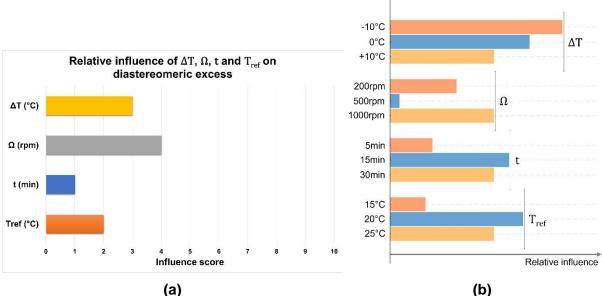
Figure E- 3: Results from Azurad for the diastereomeric excess: (a) Relative influence of the temperature difference  $\Delta T$ , the rotation speed  $\Omega$ , the residence time *t* and the reference temperature  $T_{ref}$  on the diastereomeric excess. (b) Total effect plot taken from Azurad; for every factor, the bars give the relative effect of each level to improve the diastereomeric excess.
