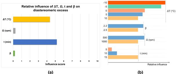
Figure E- 9: Results from Azurad for the diastereomeric excess: (a) Relative influence of the temperature difference  $\Delta T$ , the rotation speed  $\Omega$ , the residence time t and the supersaturation ratio  $\beta$  on the diastereomeric excess. (b) Total effect plot taken from Azurad; for every factor, the bars give the relative effect of each level to improve the diastereomeric excess.
