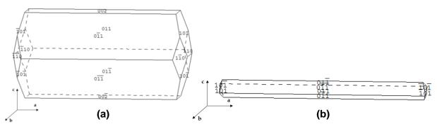
Figure II- 16: Calculated morphologies with BFDH model. (a) BFDH with distance to the central point inversely proportional to the d-spacing (1/d). (b) Variant of the BFDH model with distance to the central point proportional to exp(-Ad) with A = 0.4. Growth rate of {101} could be much faster resulting in a more extreme needle shape.
