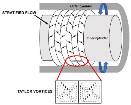
Figure I- 7: Visualization of the Taylor vortices in a CT crystallizer<sup>63</sup>.
