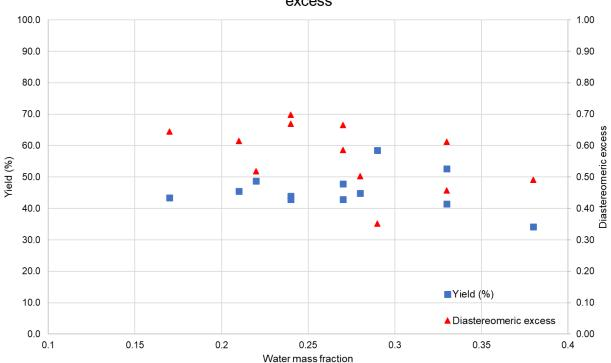
Impact of the ratio EtOH/H $_2$ O on the yield (%) and on the diastereomeric excess
