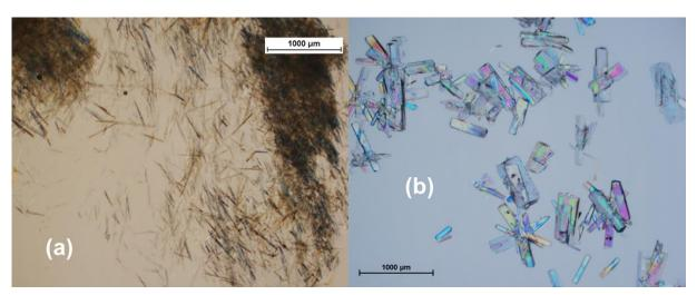
Figure II- 30: Micrographs of ss-S-Ibu-S-αMBA obtained (a) by adding the soda in technical ethanol (EtOH/H<sub>2</sub>O 95/5 w/w) and (b) by adding water without soda, taken by optical microscopy.
