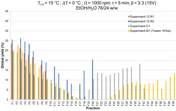
Figure IV- 27: Global yield distribution for experiments 12 R1 (orange), 12 R2 (blue), O1 (grey) and M1 (yellow). Experiment 12 R1 lasted 10 residence times, experiment 12 R2 lasted 20 residence times, experiment O1 lasted 32 residence times and experiment M1 lasted 39 residence times.
