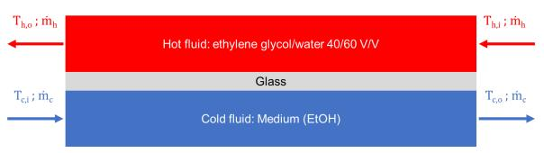
Figure III- 3: Simplified system: counter-current heat exchanger.
