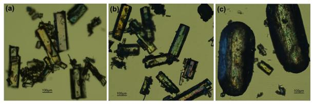
Figure IV- 19: Micrographs of the product obtained in experiment O3 (a) F1-F4: fibrous platelets, (b) F15-F19: thinner fibrous platelets and (c) F20-F48: small platelets and very big 'abraded' oblong particles, taken by optical microscopy at a magnification of 5.
