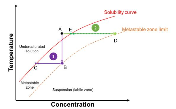
Figure I- 2: Pathways of crystallization induced by cooling (purple elements) and by evaporation (green elements).
