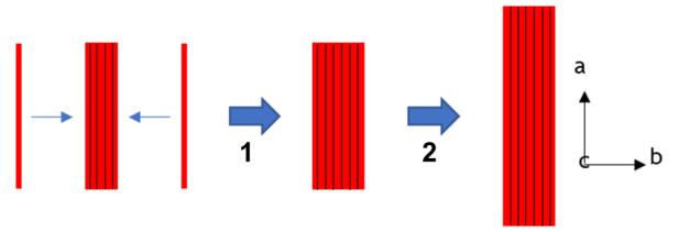
Figure II- 20: Proposition of growth mechanism for the particles of ss-S-Ibu-S-αMBA. Step 1: oriented molecular chain assembly. Step 2: Growth along the 'a' axis (main axis).
