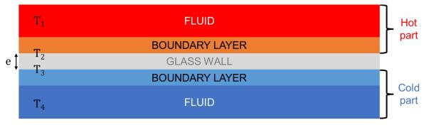
Figure III- 4: Schematic representation of the simplified system for the calculation of H.
