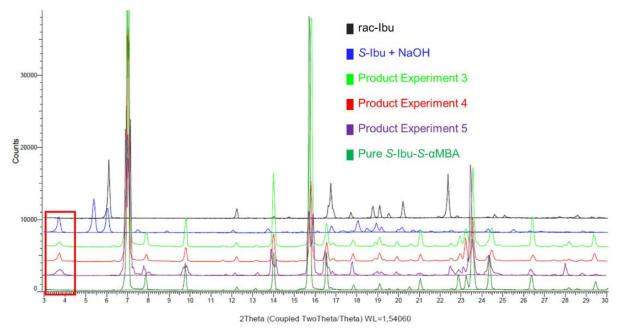
Figure IV- 9: XRPD overlay of the diffractograms of (from top to bottom): the racemic Ibuprofen (black), the product made by recrystallizing pure S-Ibu with NaOH (blue), the product of experiment B3 (light green), the product of experiment B4 (red), the product of experiment B5 (purple) and the pure S-Ibu-S-αMBA (dark green).
