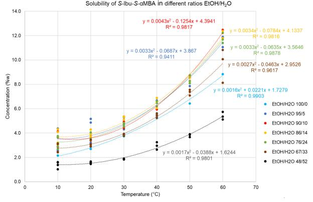
Figure II- 4: Solubility curves and polynomial trendlines of the diastereomer S-Ibu-S-αMBA in different ratios EtOH/H<sub>2</sub>O. Representation with concentration (%w) as a function of temperature (°C). Light blue ratio 100/0 w/w; dark blue ratio 95/5 w/w; red ratio 90/10 w/w; yellow ratio 86/14 w/w; green ratio 76/24 w/w; brown ratio 67/33 w/w; black ratio 48/52 w/w.
