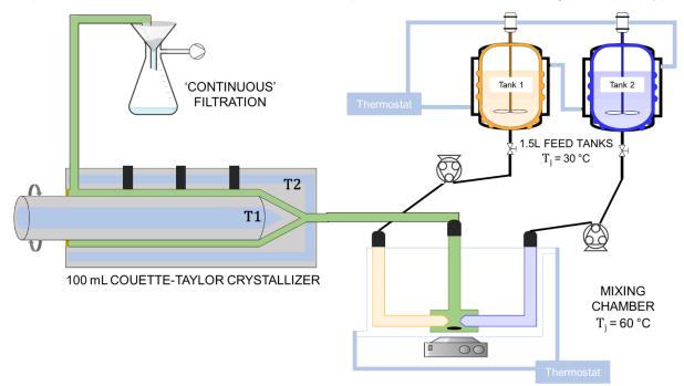
Figure III- 21: Schematic representation of the continuous set-up.
