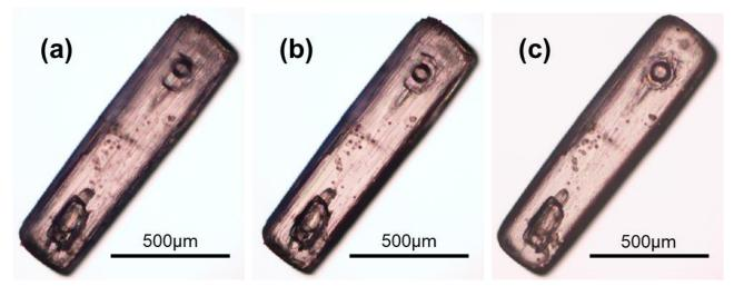
Figure II- 26: Particle of ss-S-Ibu-S-αMBA under heating (from 20 °C to 120 °C at 1 K.min<sup>-1</sup>) at three different stages: (a) at T=32 °C, (b) at T=69 °C and (c) at T=98 °C.
