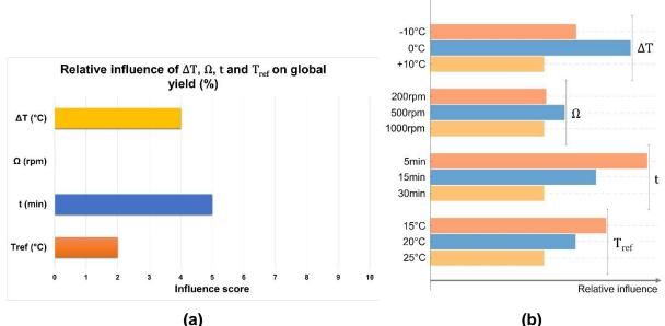
Figure E- 2: Results from Azurad for global yield: (a) Relative influence of the temperature difference  $\Delta T$ , the rotation speed  $\Omega$ , the residence time t and the reference temperature  $T_{ref}$  on the global yield. (b) Total effect plot taken from Azurad; for every factor, the bars give the relative effect of each level to improve global yield.
