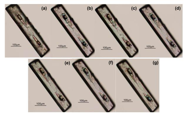
Figure II- 29: Photographs of a particle of ss-S-Ibu-S- $\alpha$ MBA undergoing the temperature cycles of Figure II- 27, extracted from the video available with the QR code of Figure II- 28. (a) t = 0 min, T = 20 °C; (b) t = 66 min, T = 80 °C; (c) t = 114 min, T = -10 °C; (d) t = 186 min, T = 80 °C; (e) t = 234 min, T = -10 °C; (f) t = 306 min, T = -10 °C; (g) t = 360 min, T = 80 °C.
