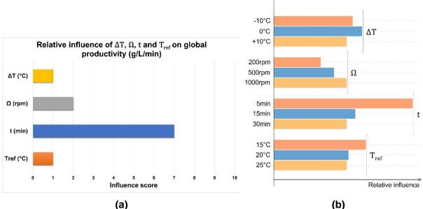
Figure E- 1: Results from Azurad for global productivity: (a) Relative influence of the temperature difference  $\Delta T$ , the rotation speed  $\Omega$ , the residence time t and the reference temperature  $T_{ref}$  on the global productivity. (b) Total effect plot taken from Azurad; for every factor, the bars give the relative effect of each level to improve global productivity.
