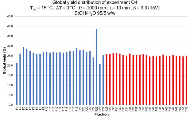
Figure IV- 20: Global yield distribution of experiment O4. The conditions are that of experiment O3, but with a solvent ratio EtOH/H<sub>2</sub>O of 95/5 w/w instead of 76/24 w/w. Blockage occurred after fraction 27. It was eliminated by heating up the CT reactor to 40 °C and flushing it with technical ethanol. Fractions 28 to 52 (red) were collected after the return of the crystallizer to the reference temperature of 15 °C.
