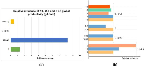
Figure E- 6: Results from Azurad for global productivity: (a) Relative influence of the temperature difference  $\Delta T$ , the rotation speed  $\Omega$ , the residence time t and the supersaturation ratio  $\beta$  on the global productivity. (b) Total effect plot taken from Azurad; for every factor, the bars give the relative effect of each level to improve global productivity.
