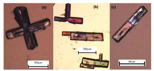
Figure II- 18: Photographs taken by binocular polarized light microscopy of the observed 'parts' of the ss-S-Ibu-S-αMBA crystals. They seem connected by a zone roughly perpendicular to the main axis 'a' of the elongated particles. (a) Particle with four visible parts; (b) and (c) particles with two or three visible parts.
