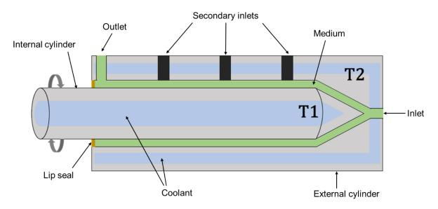
Figure III- 2: Schematic representation of the Couette-Taylor crystallizer used in this work.
