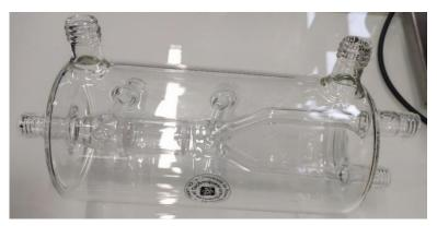
Figure III- 6: Photos of the first prototype of the temperature regulated Y-shaped connection.
