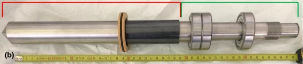
Figure III- 12: Disassembled inner cylinder. (a) view of the overheating zones and (b) view of the zones apparently not temperature-controlled (red), and temperature-controlled (green).
