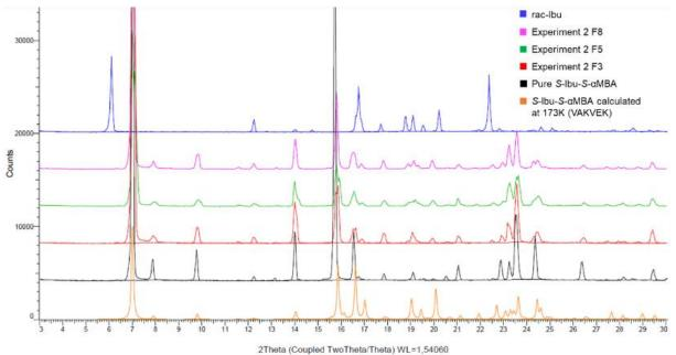
Figure IV- 14: XRPD overlay of fractions 3, 5 and 8 of experiment 2, compared with rac-Ibu, pure S-Ibu-S- $\alpha$ MBA and with the calculated diffractogram obtained from the published structure VAKVEK<sup>83</sup>.
