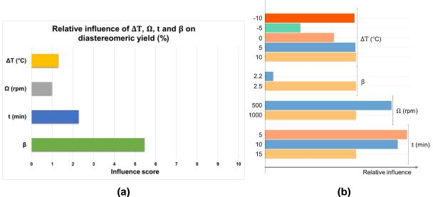
Figure E- 12: Results from Azurad for the diastereomeric yield: (a) Relative influence of the temperature difference  $\Delta T$ , the rotation speed  $\Omega$ , the residence time t and the supersaturation ratio  $\beta$  on the diastereomeric yield. (b) Total effect plot taken from Azurad; for every factor, the bars give the relative effect of each level to improve the diastereomeric yield.
