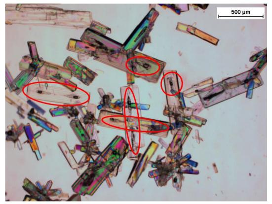
Figure II- 24: Micrograph of the product obtained in experiment B14 of Chapter IV section IV.2.1, taken by optical microscopy at a magnification of 2.5. Some fluid inclusions are encircled in red.
