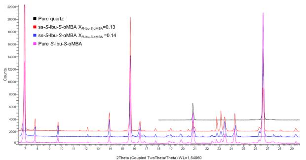
Figure II- 9: XRPD overlay of two products of partial solid solution of S-Ibu-S-αMBA (ss-S-Ibu-SαMBA) with the highest chiral purity obtained by chiral resolution of rac-Ibu, compared with pure S-Ibu-S-αMBA. Quartz was added in the sample preparation to ensure an internal calibration of the diffractograms on the peak 26.6 °20.
