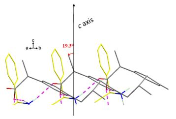
Figure II- 10: Inclination of the bond C\*-C with reference to the c-axis.
