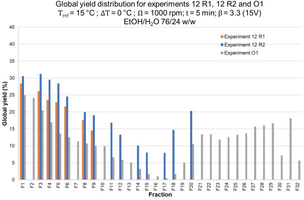
Figure IV- 16: Global yield distribution for experiments 12 R1 (orange), 12 R2 (blue) and O1 (grey). Experiment 12 R1 lasted 10 residence times, experiment 12 R2 lasted 20 residence times and experiment O1 lasted 32 residence times.
