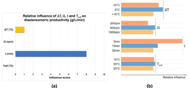
Figure E- 4: Results from Azurad for the diastereomeric productivity: (a) Relative influence of the temperature difference  $\Delta T$ , the rotation speed  $\Omega$ , the residence time t and the reference temperature  $T_{ref}$  on the diastereomeric productivity. (b) Total effect plot taken from Azurad; for every factor, the bars give the relative effect of each level to improve the diastereomeric productivity.
