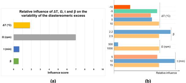
Figure E- 10: Results from Azurad for the standard deviation of the diastereomeric excess: (a) Relative influence of the temperature difference  $\Delta T$ , the rotation speed  $\Omega$ , the residence time t and the supersaturation ratio  $\beta$  on the variability of the diastereomeric excess. (b) Total effect plot taken from Azurad; for every factor, the bars give the relative effect of each level on the variability of the diastereomeric excess.
