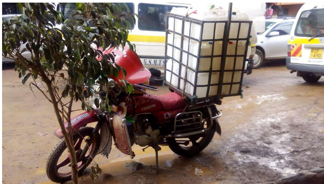
Figure 3.23: Fabricated motorbike with a capacity of about 200 litres of milk.
