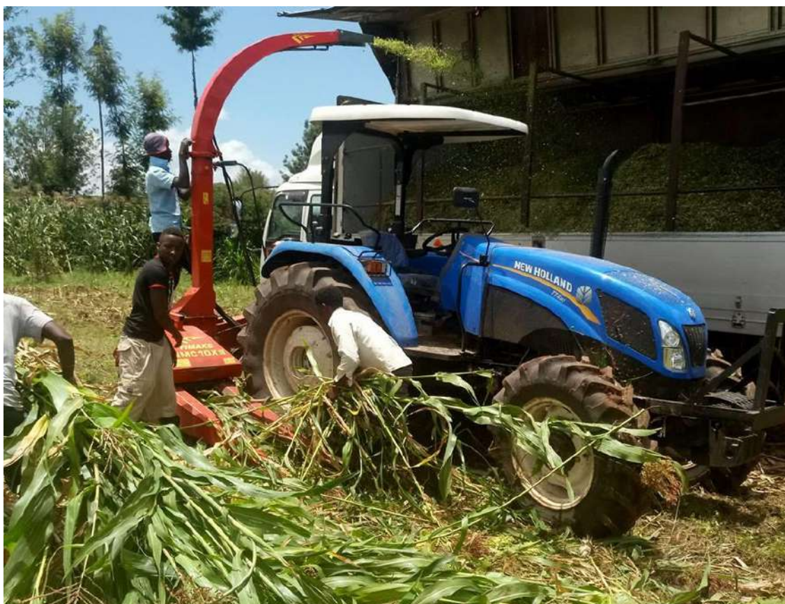
Figure 3.12: Harvesting of fodder using a silage chopping machine.
