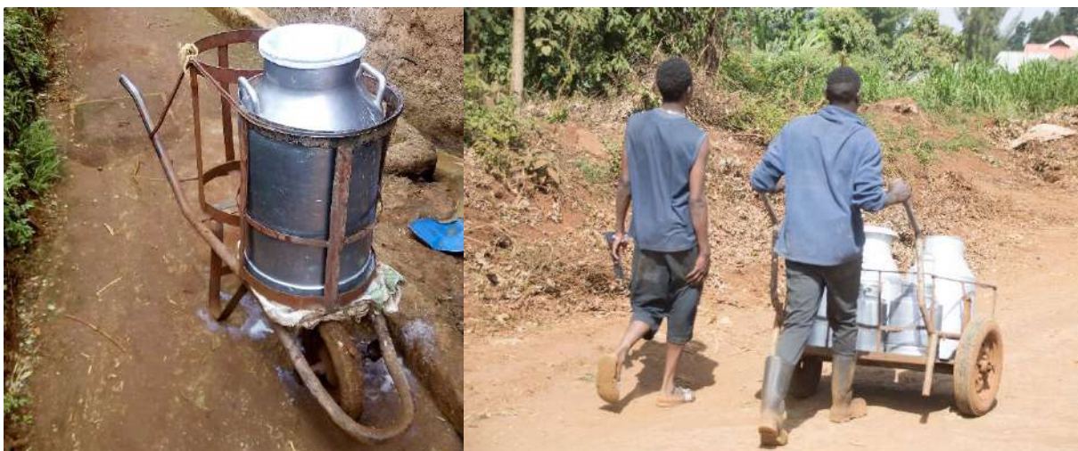
Figure 4.14: Modified wheelbarrow and handcart.
