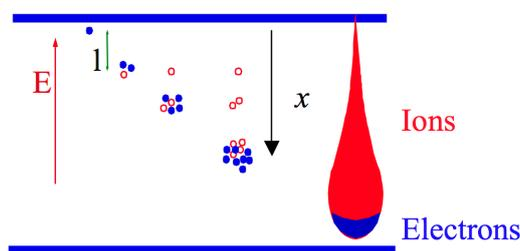
Figure 2.14: Charge multiplication in a uniform field.  $l = \lambda$  is the mean free path for ionization [19].
