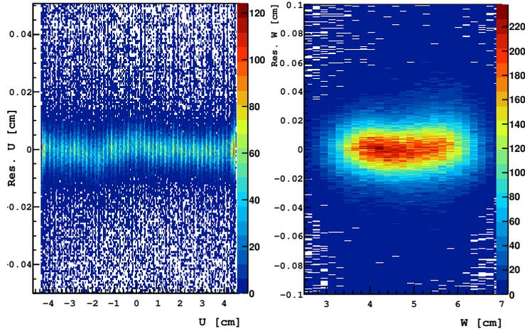
Figure 6.9: Evolution of residuals along the measured coordinate for U and W. The fluctuations at  $W \approx 4.6$  cm and  $U \approx -0.2$  cm indicates a local field distortion in the middle of the TPC. U and W are correlated via the beam geometry.
