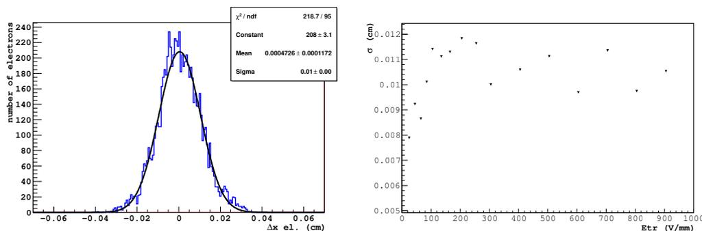
Figure 9.7: [Left] Distribution of the distance between the position of the primary electron and the position of the electrons in the readout plane. [Right] Evolution of the  $\sigma$  of the fitted Gaussian function of the [Left] distribution versus the transfer field.
