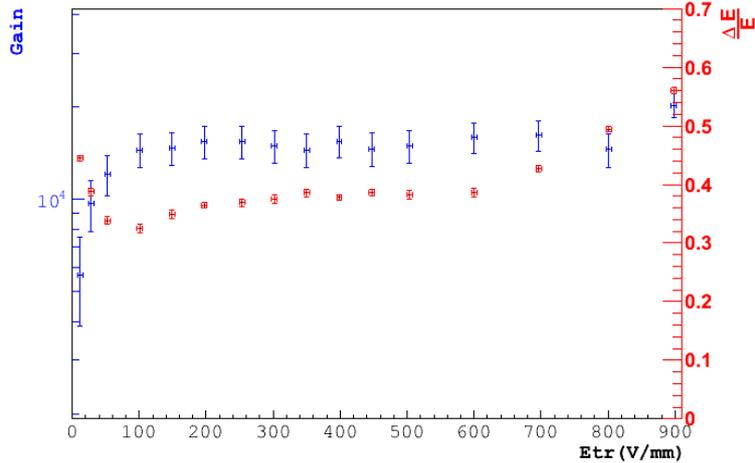
Figure 8.9: Gain and  $\frac{\Delta E}{E}$  for TF10V2-04 (standard bulk + GEM with a gap of 1 mm) for different transfer fields. Large errors on gain are due to the uncertainty on the GEM voltage that is multiplied by the gain of the mesh. The drift field is set at 800 V/cm,  $V_{\text{MESH}} = 280$  V and  $V_{\text{GEM}} = 300$  V.
