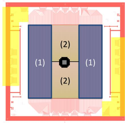
Figure 10.1: Schematics of the Pixel Micromegas detector. The zone labeled (1) is segmented into 40 cm long strips at a pitch of  $480\ \mu\text{m}$ , and (2) of 20 cm long strips at a pitch of  $400\ \mu\text{m}$ . The pixelized area in the center of the detector is divided between the 6.25 mm long pixels, in black, and the 2.5 mm long pixels in gray. Connectors highlighted in yellow are connected to the pixels, the others (in pink) to the strips.
