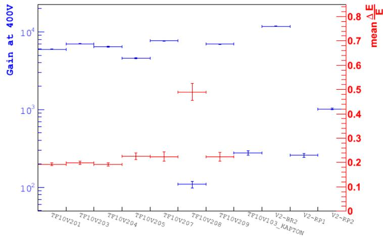
Figure 8.10: Summary of gain and energy resolution measurements at  $V_{\text{MESH}} = 400\text{V}$  for the TF10 Micromegas prototypes. V2-BR2, V2-RP1 and V2-RP2 are the values for TF10V2-BR2, TF10PI-RP1 and TF10PI-RP2.
