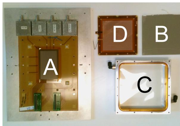
Figure 8.3: The different part of a standard prototype with a GEM foil. A: PCB mounted on an aluminum frame. B: the  $25 \mu\text{m}$  aluminized Mylar drift electrode. C: gas vessel aluminum frame and Mylar window. D:  $10 \times 10 \text{ cm}^2$  gem foil
