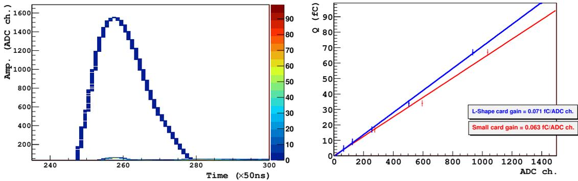
Figure 4.4: [Left] a typical pulse recorded by the AFTER-T2K FEE. The shaping time has been lowered to  $\tau_p = 1000$  ns to have more measurement points with a 20 MHz clock. [Right] Data points and linear fit of the gain calibration for the two different front-end cards. This calibration is viable for the parameters used with the test-chamber ( $\tau_p = 100$  ns, 120 fC charge range).
