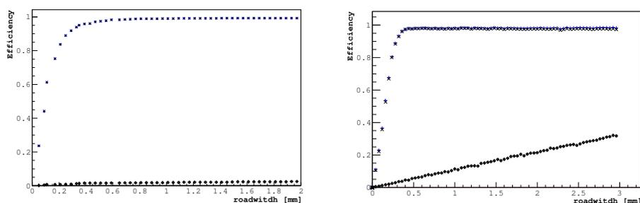
Figure 8.13: [Left] Evolution of the raw efficiency (black crosses), corrected efficiency (blue  $\times$ ) and background probability (black  $+$ , almost superposed to the blue  $\times$ ) on TF10V2-03. [Right] Monte-Carlo simulation of a 98% efficiency detector with one background cluster for each event.
