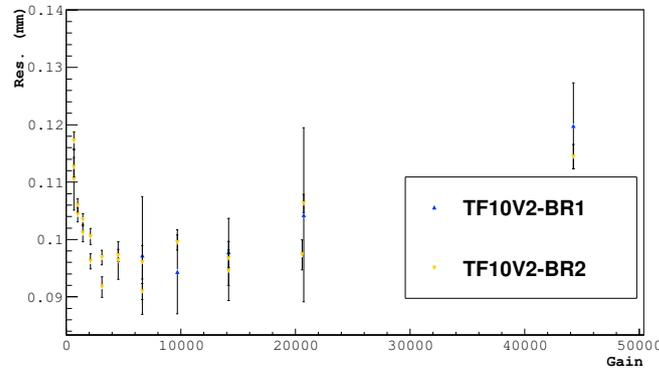
Figure 8.20: Evolution of the resolution of the TF10-BR1 and TF10-BR2 detectors with gain.
