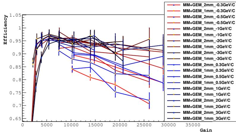
Figure 8.25: Efficiency versus gain for various momentum for GEM-Micromegas with a 0.2 to 3 GeV/c hadron beam. Blue lines represent positive hadrons and red is for negative.
