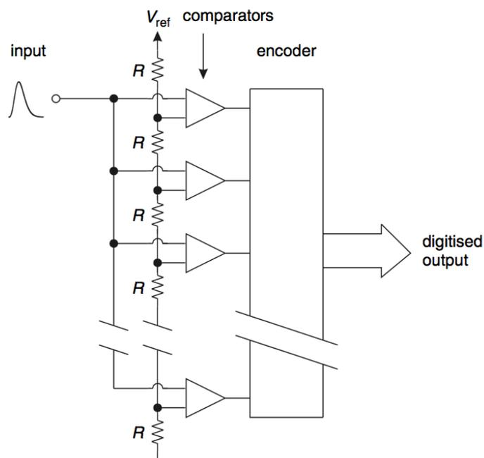
Figure 2.22: Principle of a flash ADC. “input” is compared to the reference voltage  $V_{ref}$  and its division by powers of two by the comparators. When “input”  $>$   $V_{ref}$ , the overflow signal is at ‘1’. The ADC is synchronized with a clock signal that enables the encoder to convert its input into bits [35].
