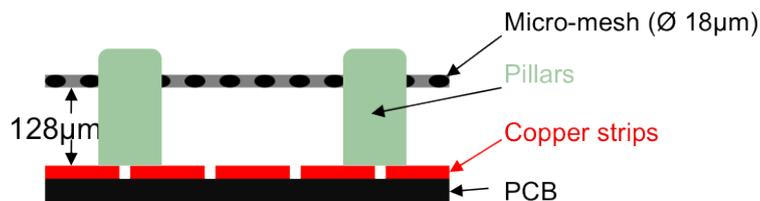
Figure 2.6: Principle of the bulk Micromegas. The woven micro-mesh, after lamination, is embedded into insulator pillars on the readout PCB. See also Fig. 2.7.
