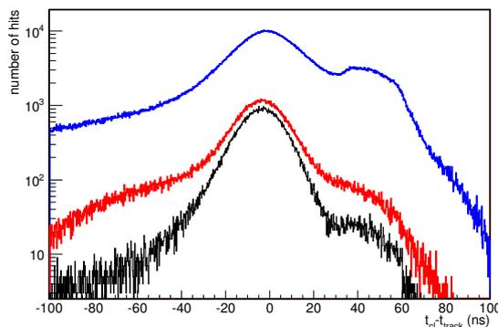
Figure 10.18: Effect of the different cuts on the time distribution of PMM\_GEM\_2011\_2. The blue curve is the distribution with no selections on tracks. The red curve includes only the clusters inside the road width around the tracks. The black line corresponds to the same distribution when only tracks belonging to a primary vertex are considered.
