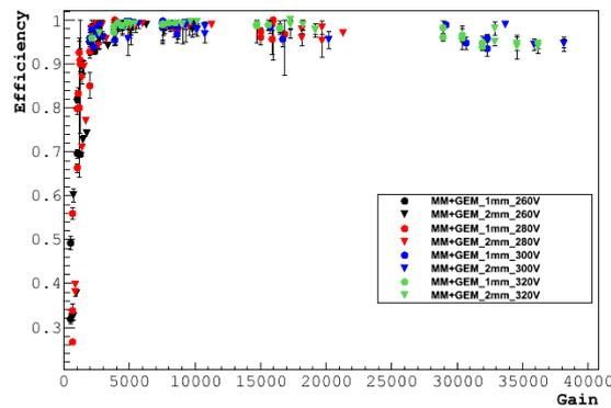
Figure 8.15: Background corrected efficiency of the two GEM-Micromegas detectors. The colors of the symbols represent different gains of the GEM foil corresponding to a  $\Delta V_{\text{GEM}}$  from 260 to 320 V.
