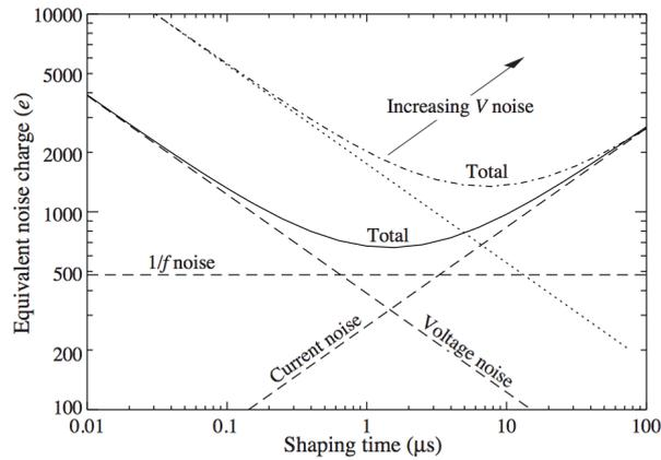
Figure 2.32: ENC in function of the shaping time  $\tau$ . At small  $\tau$ , voltage noise is dominating; at large  $\tau$  it is the current noise. This creates an optimal ENC when the voltage noise equals the current noise. The  $1/f$  noise is independent of the shaping time. An increase of the voltage noise increases the optimal  $\tau$  [48].
