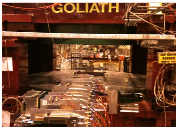
Figure 8.12: The 12 detectors on the test bench at the H4 beam line of the SPS in front of the GOLIATH magnet.
