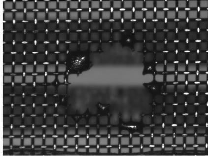
Figure 7.6: Microscope view of a damaged bulk micro-mesh after an important discharge.
