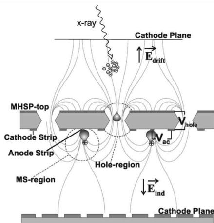
Figure 2.10: MHSP schematic diagram and its operating principle [20]. Charges deposited above the MHSP by radiation, *e.g.* an X-ray photon, are focused into a hole and multiplied as in a GEM. Avalanche electrons are transported toward the anode strips and multiplied in a second avalanche process. A part of the avalanche ions are collected at the cathode plane localized below the MHSP.
