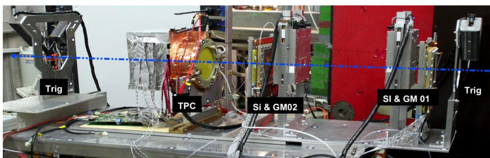
Figure 6.1: Test bench at the ELSA facility, the dashed blue line represents the electron beam. Along the beam direction, from right to left : (Trig) First trigger station; (SI & GM 01 and 02) First and second silicon stations and GEM detectors 01 and 02; (TPC) GEM-TPC test chamber with its FEE protected with EM shielding; (Trig) last trigger station.
