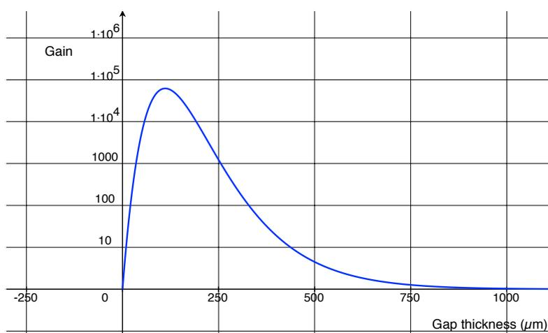
Figure 7.5: Evolution of the gain (in log) of a parallel plate detector with respect to the amplification gap thickness. Eq. 7.1 in Ar/ $i\text{C}_4\text{H}_{10}$  95/5 with  $A = 3 \times 10^3 \text{ m}^{-1} \text{ kPa}^{-1}$ ,  $B = 6 \times 10^3 \text{ m}^{-1} \text{ kPa}^{-1}$  (from [76]),  $P = 90 \text{ kPa}$  and  $V_{\text{MESH}} = 60 \text{ V}$ .
