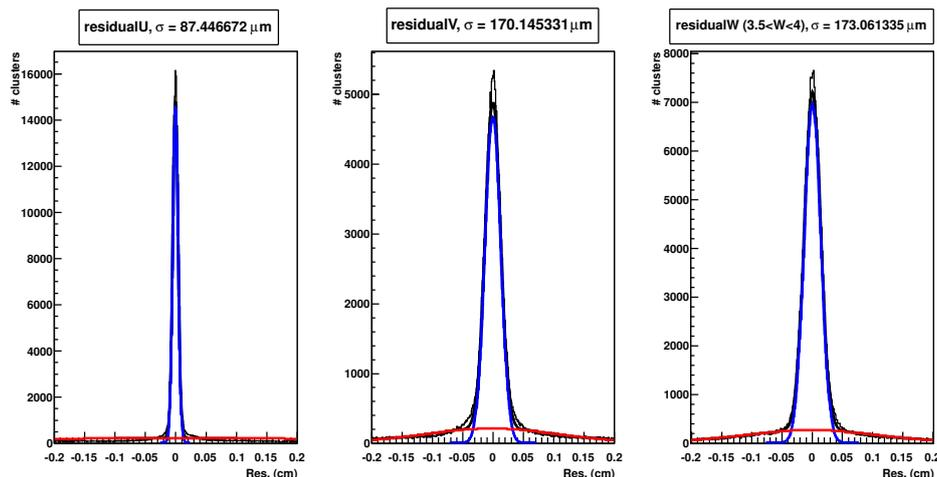
Figure 6.8: Biased residuals between the test chamber clusters and internally reconstructed track, projected in detector coordinates. Only the 1.25 mm pads are used here. Residuals are fitted with a sum of 2 Gaussians (black line) composed of a large Gaussian (red) and a narrow one (blue).  $\sigma$  is the weighted mean of the red and blue Gaussians for each projection. Fit errors are below  $1 \mu\text{m}$ .
