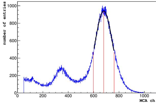
Figure 8.5: Spectrum of  $^{55}\text{Fe}$  in  $\text{Ar}+5\%i\text{C}_4\text{H}_{10}$  for the TF10V2-06 prototype. The 3 keV and 5.9 keV peaks can be seen. The second peak is fitted with a Gaussian (in black), reconstructed maximum ( $E$ ) and FWHM ( $\Delta E$ ) from the fit parameter are shown with the red vertical lines.
