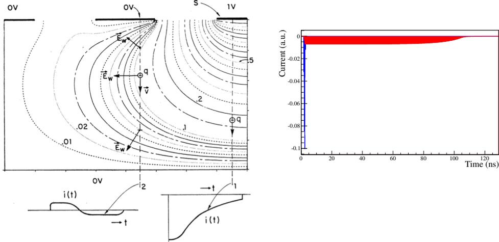
Figure 2.15: Left: The induced signals on strip by two charges using the weighting field  $\vec{E}_w$  of the right strip at 1 V [5]. Right: Garfield simulation of an induction signal in a Micromegas strip detector, see Chap. 9. Blue represents the part of the signal induced by electron, red by ions.
