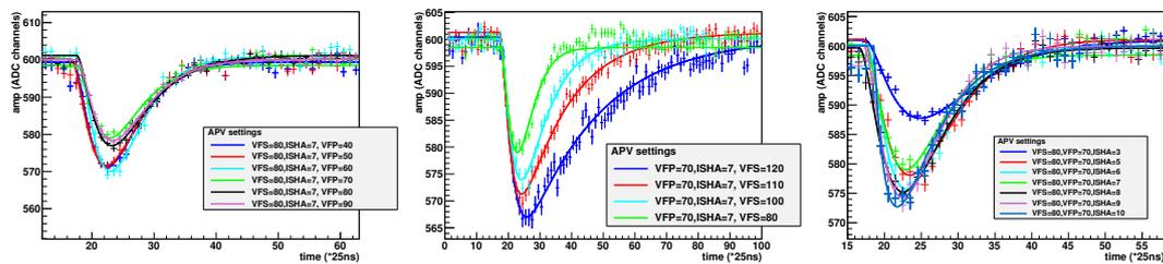
Figure 10.6: Influence of, from left to right, VFP, VFS and ISHA on the APV signal shape. VFS influences the decay length of the tail, ISHA the rising time and VFP the pre-amplifier gain which is hidden by the shaper that comes later in the APV processing chain.
