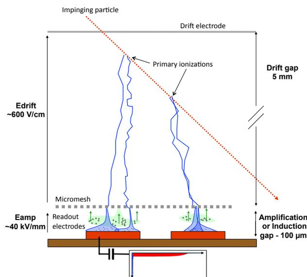
Figure 7.3: Principle of the Micromegas detector.
