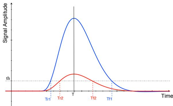
Figure 2.30: Effect of time walk: for two signals that have the same timing but not the same amplitude, rising and falling times ( $T_r$  and  $T_f$ ), at a certain threshold  $th$ , show non linearity with respect to the time  $T$ .
