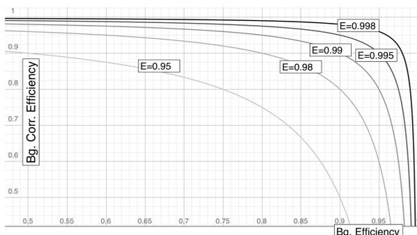
Figure 10.7: Evolution of the corrected efficiency with the background efficiency for different values of apparent efficiency. The evolution of the correction depends on the apparent efficiency  $E$  of the detector. A detector with a 99.8% uncorrected efficiency can sustain 60% background efficiency without significant loss.
