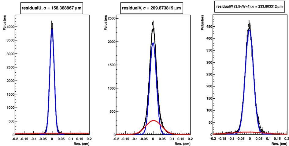
Figure 6.10: Residuals between test chamber cluster and tracks reconstructed by the telescope projected in the TPC coordinates. Residuals are fitted with a double Gaussian (black line) composed of a large Gaussian (red) and a narrow one (red).  $\sigma$  is the weighted mean of the red and blue Gaussians for each projections. Fit errors are below  $1 \mu\text{m}$ .
