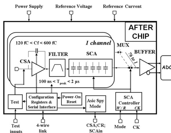
Figure 4.1: Internal architecture of the AFTER ASIC. From [39].
