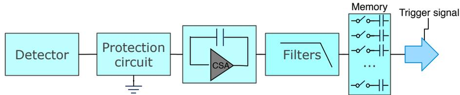
Figure 2.17: Front-end electronics chain from detector to digitization.
