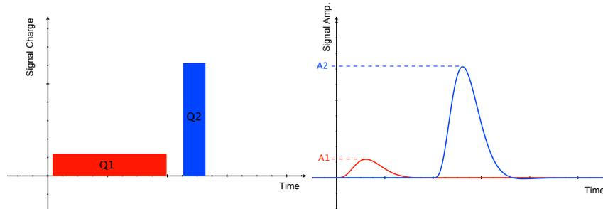
Figure 2.28: Effect of ballistic deficit, the same original charge,  $Q_1 = Q_2$ , leads to two different amplitudes  $A_1 \neq A_2$  after shaping because of two different rising times.  $Q_1$  typically represents a signal that had more diffused than  $Q_2$ .
