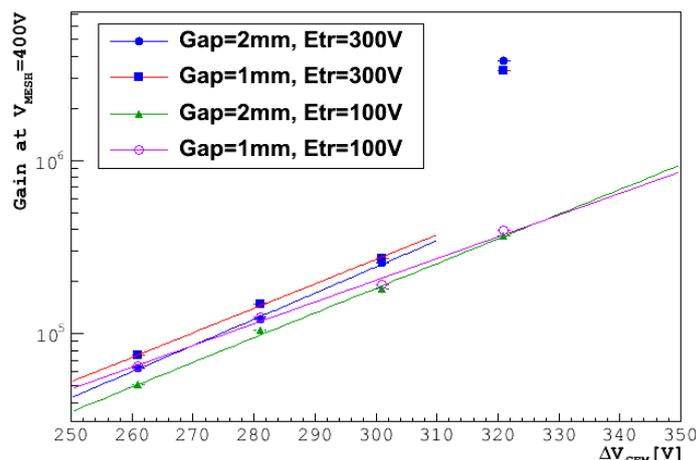
Figure 8.8: Gain of the GEM-Micromegas prototypes for different  $\Delta V_{\text{GEM}}$ . The values are an extrapolation of the fit of the gain function at  $V_{\text{MESH}} = 400$  V. Errors include errors on data points of  $G(V_{\text{MESH}})$ , fit errors and HV settings uncertainties.
