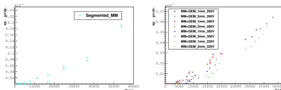
Figure 8.21: Discharge probability of the segmented Micromegas [Left] and GEM-Micromegas [Right] detectors with respect to the detector gain. These measurements are done with the SPS beam of the 2010 RD51 beam period, *i.e.* hadrons (80%) and muons (20%) at 170 GeV/c.
