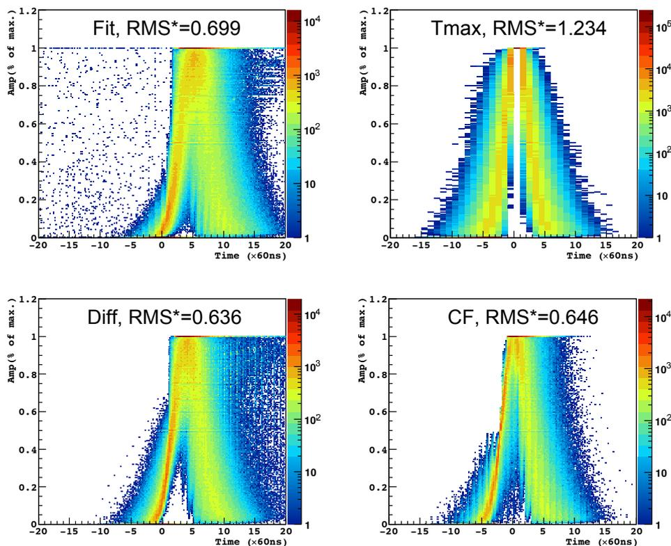
Figure 5.8: Superposition of normalized signals from krypton data, shifted at the different reconstruction signal time, see text. The “RMS\*” is computed for the rising edge (left leg of the signal) between 0.18 and 0.22.
