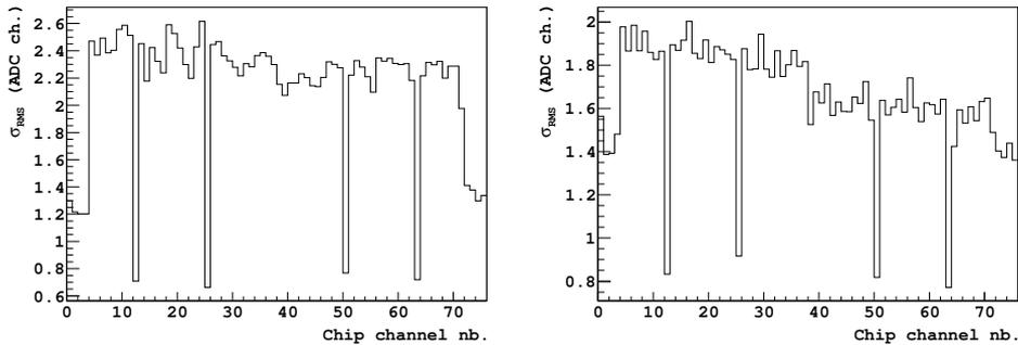
Figure 4.6: Noise spectrum of one ASIC of the L-shape [Left] and small [Right] FEC. For the L-card ASIC, the noise is  $1.94 \pm 0.11$  ADC channels on connected channels (the error is the RMS of the noise distribution). The small card has a noise of  $1.58 \pm 0.05$  ADC ch. The spectrum shows a division between the first and second half of the ASIC that are connected to a different side of the packaging, their noise levels are respectively  $1.55 \pm 0.10$  and  $1.63 \pm 0.06$  ADC ch. .
