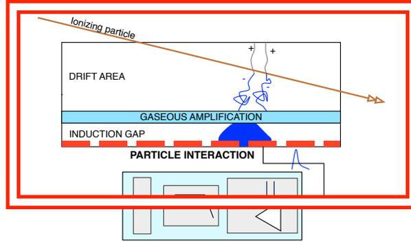
Figure 2.13: Drift of primary electrons and formation of an electrical signal on the detector electrodes.
