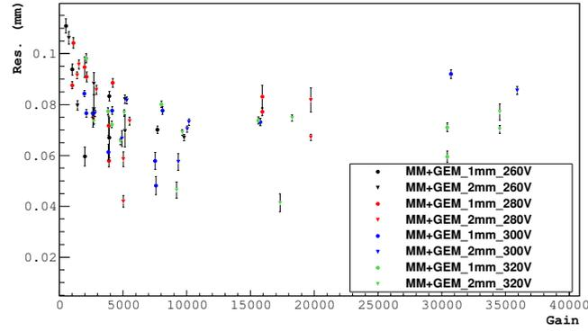
Figure 8.19: [Left] Resolution of the GEM-Micromegas detectors with respect to the detector gain. The colors of the symbols represent different gains on the GEM foil corresponding to a  $\Delta V_{\text{GEM}}$  from 260 to 320 V.
