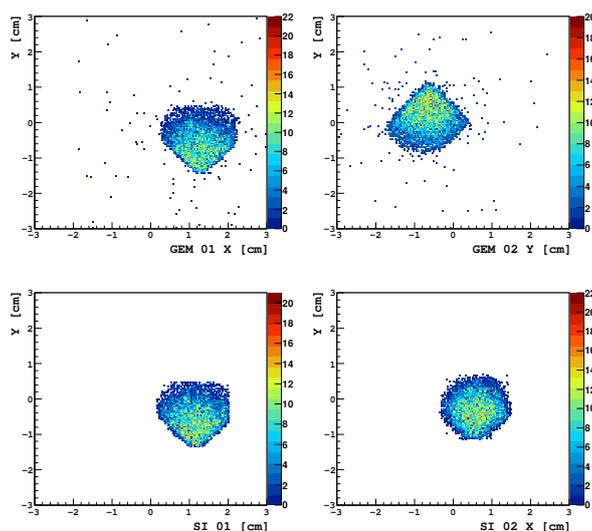
Figure 6.4: Hit position of the tracking detector clusters for 10000 events with a reconstructed track ( $\sim 72\%$  of all events). The angle of the halo beam with respect with the trigger acceptance appears.
