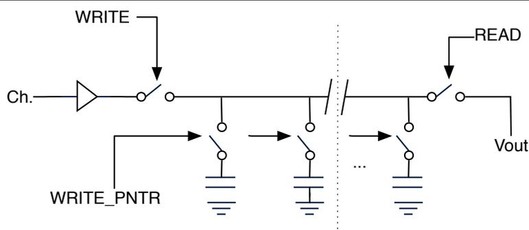
Figure 2.21: Principle of an analog memory: the Switched Capacitor Array (SCA). The signal “WRITE” connects a channel to the storing capacitor connected by the signal “WRITE\_PNTR”. When the values need to be read, the “READ” signal connects the memory cell to Vout.
