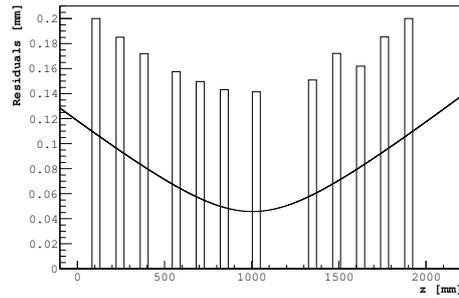
Figure 8.17: Width of the residual distribution along the Z axis for each detector (vertical bars). The plain line represents the analytical formula of Eq. 8.5. The spatial resolution for the reference detector is  $80\ \mu\text{m}$ .
