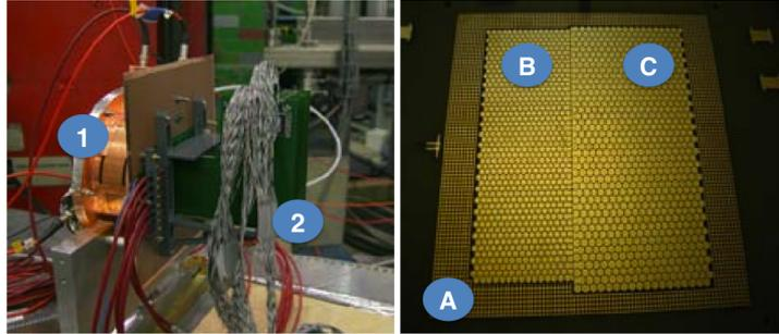
Figure 3.2: [Left] The GEM-TPC test chamber (1) and its electronics (2). [Right] Inside the test chamber, the  $10 \times 10 \text{ cm}^2$  active area which is divided between (A) grid at ground potential to homogenize the induction field, (B) 1.25 mm hexagonal pads and (C) 1.5 mm pads.
