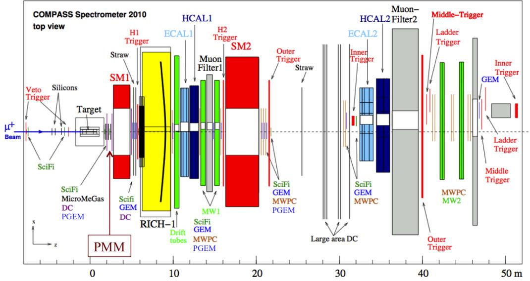
Figure 7.1: Top view of the COMPASS spectrometer setup in 2010 with the PMM prototype position at  $\sim 2$  m from the target, in between Micromegas detectors. Picture taken from [70].
