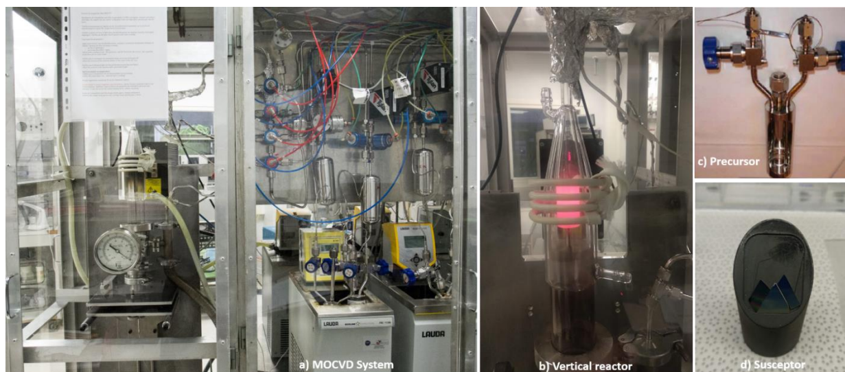
Figure 2.7: These images depict all the lines and equipment (valves, mass flow meters, connection lines, bubblers...), ensuring the transport of active gases toward the reactor and get growth. The gas lines are stainless steel tubes electropolished on the inside with low roughness to limit the memory effect. The components are connected to the lines by means of metal gaskets serving as fittings, ensuring a good seal. The substrates are placed on the susceptor before introduction in the reactor.
