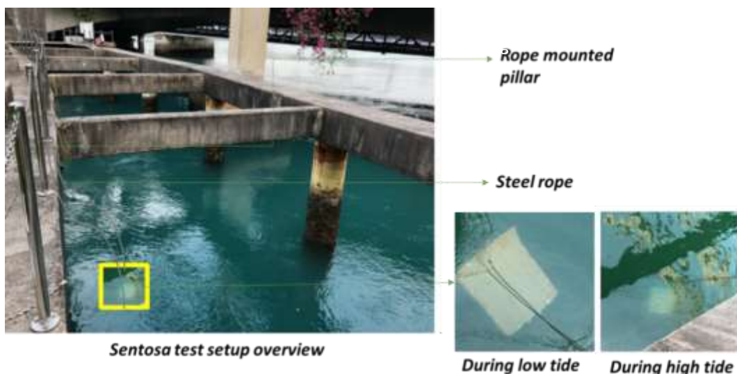
Figure 10: Immersion test facility at NTU Singapore.
