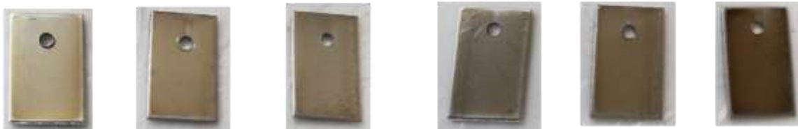
Figure 5: Naked-eye observation of coated sample before and after 120 h of immersion in 3.56 wt.% NaCl solution
