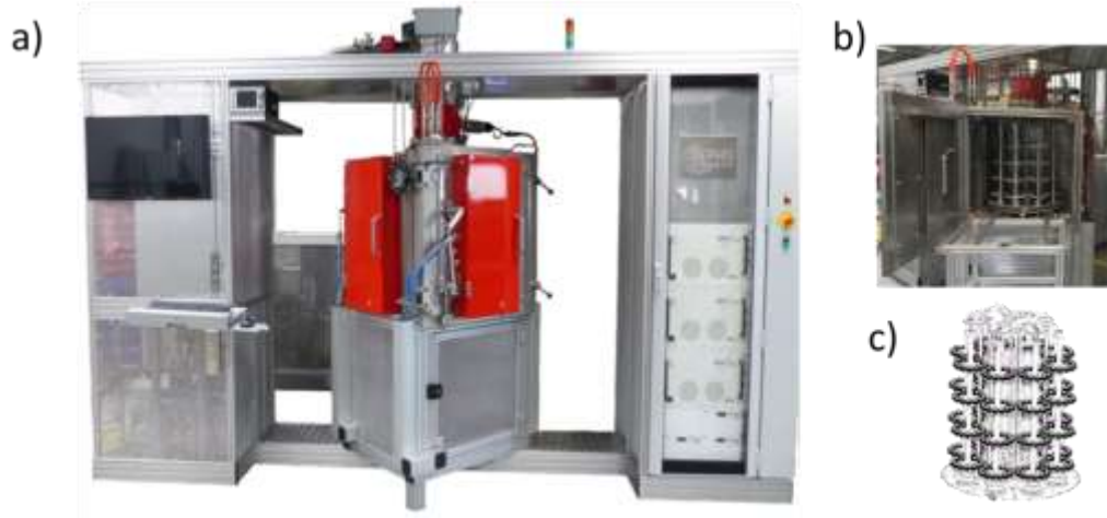
Figure 2: Photographs of the a) inside, b) outside of TriPros reactor and c) drawing of the substrate-holder.
