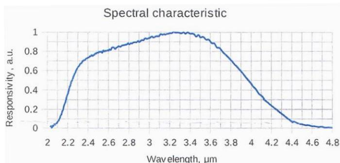
**Figure 4.8** Responsivity of mid-infrared photomixer
