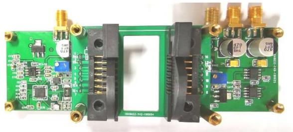
**Figure 3.7** Physical map of homemade DFB laser control circuit
