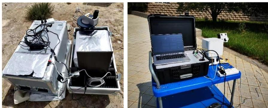
**Figure 3.1** (a) Device of EM27/SUN; (b) Device of IP-NIR-LHR
