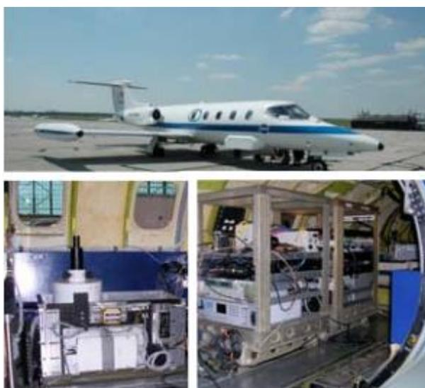
**Figure 5** Aircraft equipped with lidar <sup>[13]</sup>
