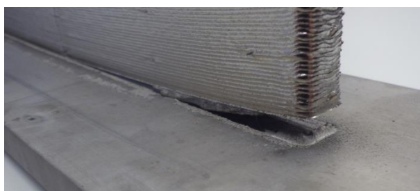
Figure 1. 10: Warping leading to build-part's detachment from the substrate/base-plate (Irepa Laser: AMAZE Project)
