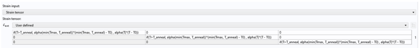
Figure 4. 7: Implementation of elastic strain contribution with relaxation condition as external strain feature in COMSOL
