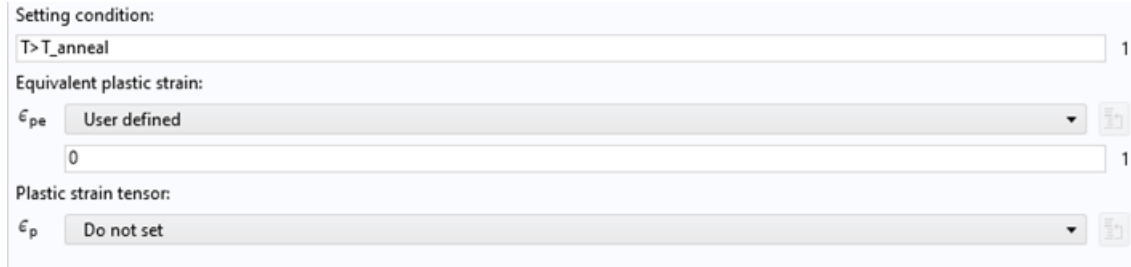
Figure 4. 6: Implementation of equivalent plastic strain condition in COMSOL that removes the deformation history by re-setting the yield surface to the on-set of plasticity of the material
