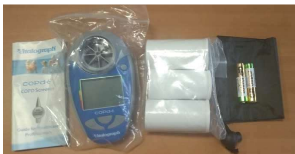
Plate 2: Portable digital spirometer, disposable mouthpieces and batteries used to conduct Spirometry assessment in communities, Kano State, Nigeria.
