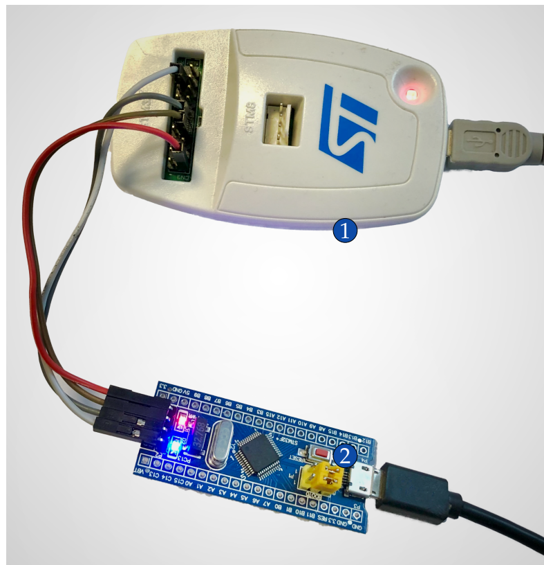
Figure 4.3 – Hardware keyboard emulator bait consists of one Blue Pill STM32 board ① connected to a ST-link v2 ② which under control of ULTRA host agent.
