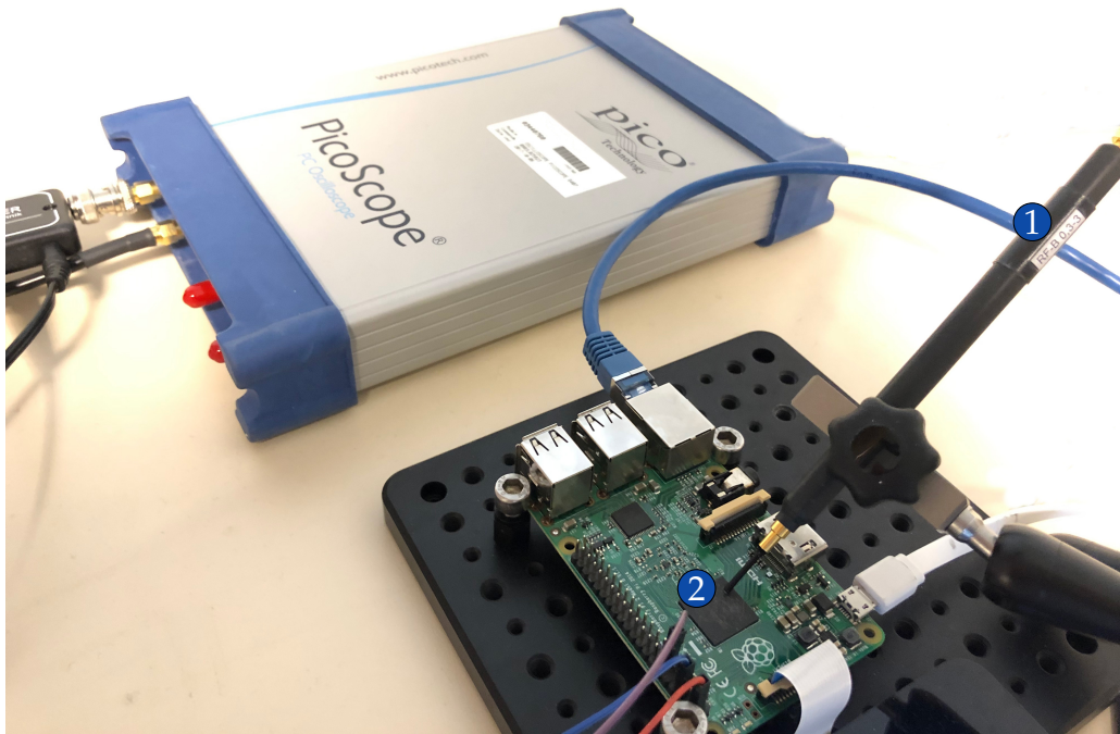
Figure 3.4 – Probe setup consists of a H-Field probe ① placed 45 degree above the Raspberry Pi processor ②.
