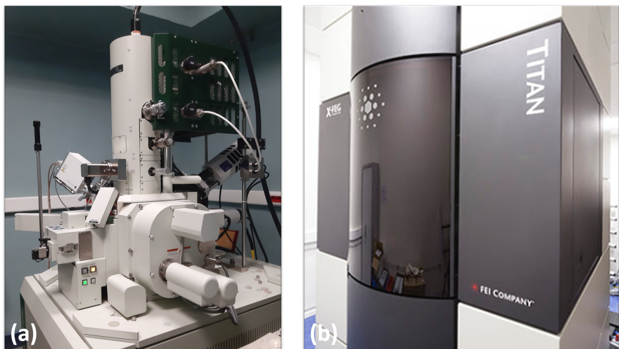
Figure 2.17: (a) JEOL JSM-7800F scanning electron microscope; (b) Thermo Fisher Scientific™ Titan Themis
