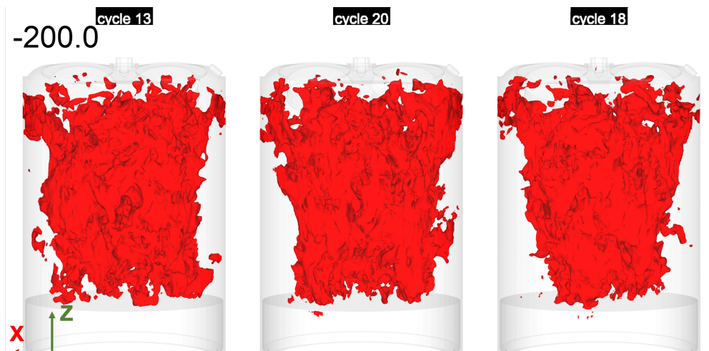
FIGURE 7.16: Intake jet at -200 CAD, visualized by iso-surface of U_z = -10 m/s. View from the exhaust side.
