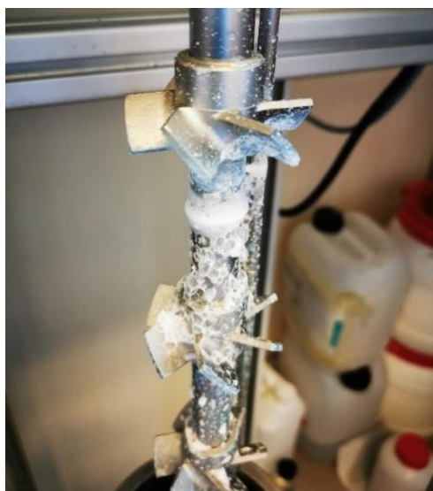
Figure 3.5 Material deposited on the shaft after the semi-batch reaction S075.153.11.120.
