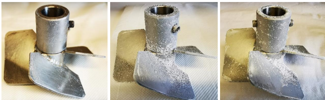
Figure 4.24 Bottom and side views of the material attached to the hydrofoil after the semi-batch reactions at different CTA concentrations a) 15.3 g/L, b) 7.8 g/L A and c) 7.8 g/L B.
