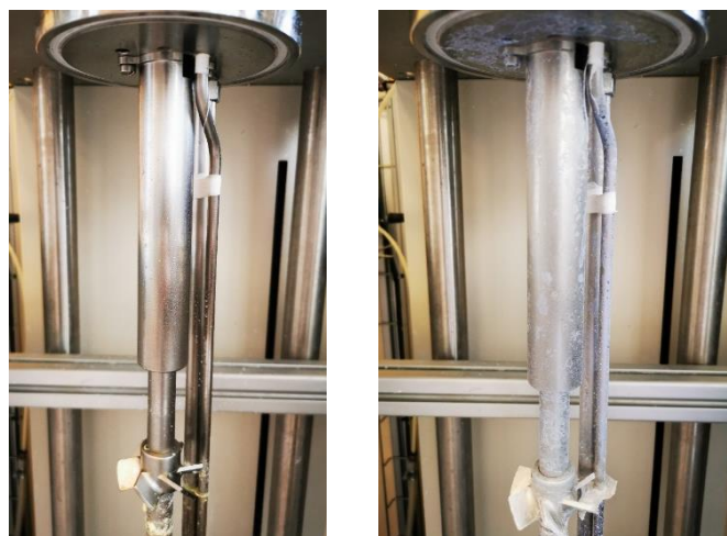
Figure 4.26 Fouling on the head of the reactor after a semi-batch reaction with depressurization rate of a) 8 bars/min and b) 2 bars/min.
