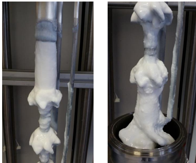
Figure 3.7 View of the material deposited on the impellers after 100 minutes at 83 °C and 550 rpm.
