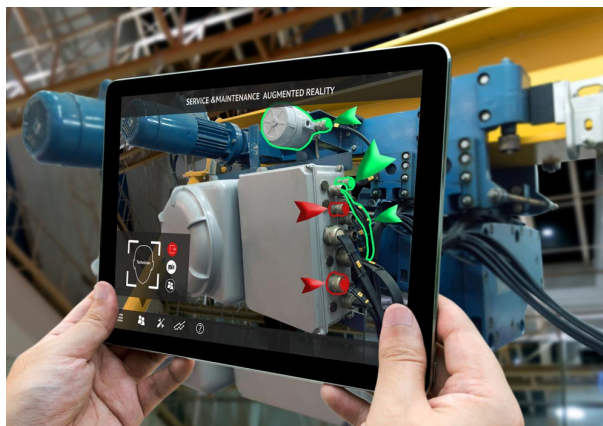
Figure 2 – Example of augmented reality application for the industry, where virtual content is attached to an object. Image courtesy of ptc-solutions.de .
