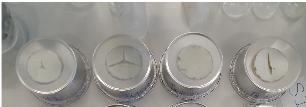
Figure. S5 : Deposited self-supported films prepared for tensile strength measurements. Numerous deposits had a broken structure after drying at room temperature.
