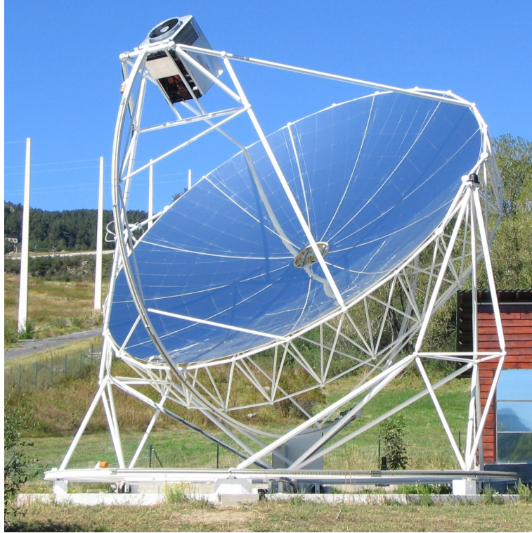
Figure 1.5: PROMES's 10 kW Dish-Stirling system (Odeillo, France).
