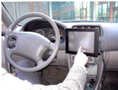
FIGURE 2.14. The touch screen used for the secondary task mounted in the instrumented vehicle in both [41, 132] studies. Image reproduced from [41]
