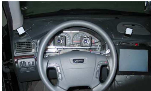
FIGURE 2.15. Face LAB cameras mounted behind the steering wheel in order to record eye movements. Image reproduced from [41]
