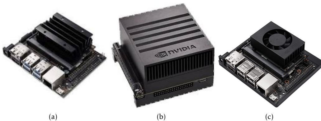
Figure 6.2: (a) Nvidia Jetson TX1 (b) Nvidia Jetson Xavier AGX (c) Nvidia Jetson Xavier NX
