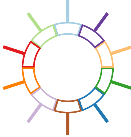
Figure IV.2 – Representation of a cyclic structure with sector mistuning as introduced with the IMM method.
