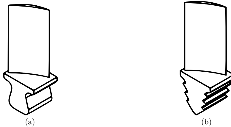
Figure I.7 – Schematic representation of (a) a dovetail root and (b) a fir tree root [JetX Engineering].
