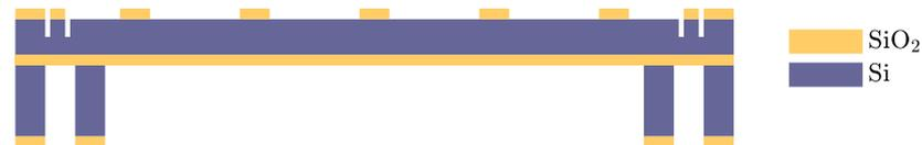
Figure 4.24: Top wafer after the back cavity etching
