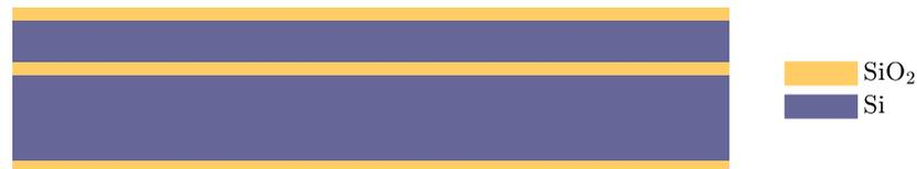
Figure 4.1: Bottom wafer
