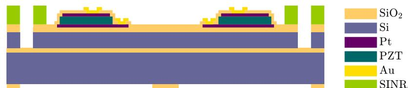
Figure 4.15: Bottom wafer after the deposition and patterning of the SINR glue
