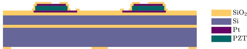
Figure 4.8: Bottom wafer after deposition and etching of the passivation layer
