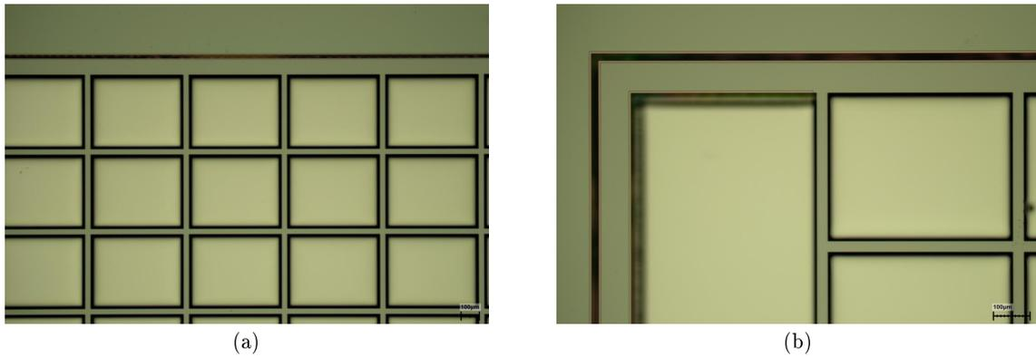
Figure 4.28: Microscope picture of the top wafer after the etching of the stiffeners (a) and zoom around the linearization spring (b)
