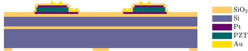
Figure 4.9: Bottom wafer after deposition and etching of the metal pads
