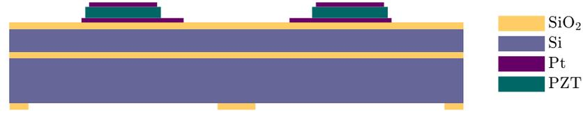
Figure 4.5: Bottom wafer after etching of the PZT stack
