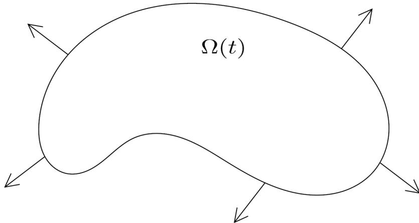
Figure 1.7 – The moving domain  $\Omega(t)$ . The arrows represent the velocity vector defined by  $v = (-\nabla p \cdot \vec{\nu})\vec{\nu}$  on  $\partial\Omega(t)$ .
