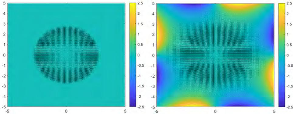
Figure 1.6 – Curl  $v$  (colorbar) overlapped with the vector  $v$  (arrows in black). Left: Darcy's law with  $\kappa = 1$ . Right: Brinkman's law with  $\mu = \kappa = 1$  and Dirichlet boundary conditions. The pressure is taken as :  $p(x, y) = 10^3 e^{-1/(1-(x/3)^2-(y/3)^2)} \chi_{(x/3)^2+(y/3)^2 \leq 1}$ , with  $\chi$  the indicator function.
