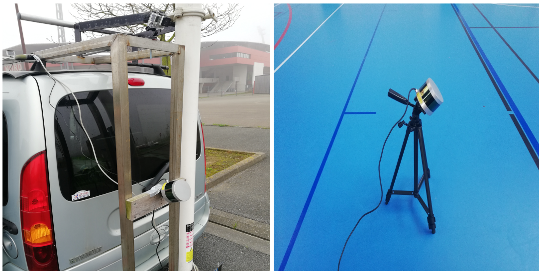
(a) VLP-16 LiDAR mounted on a vehicle (b) VLP-16 LiDAR mounted on a fixed stand
