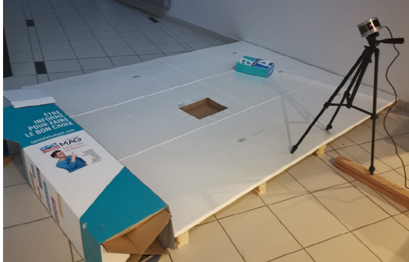
FIGURE 5.24: Acquisition of hump and pothole defects
