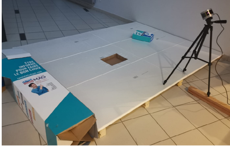
FIGURE 5.24: Acquisition of hump and pothole defects
