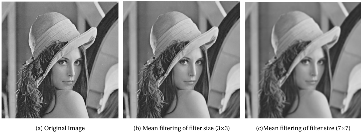
Figure 2.12: Example of mean filtering result with different filter size
