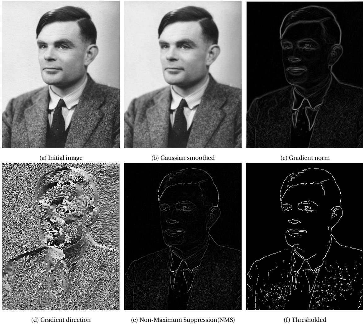
Figure 2.18: Example of Canny edge detection implementation and result
