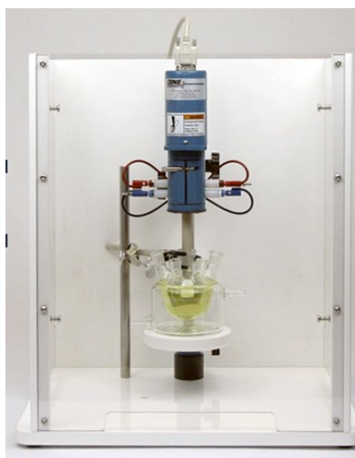
Figure 3-23. Cyclic voltammetry setup in a homemade glass electrochemical cell.
