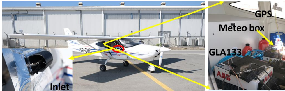
Figure S1.1 The setup of the airborne measurement system.
