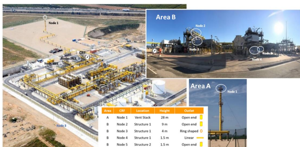
Figure 3.1 Aerial view of the Enagas site in Spain and node placement (white circles). The controlled release facility is indicated by a white disk marked “CRF”.
