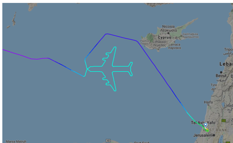
Figure 1.3: A typical anomalous emission of ADS-B data resulting in a plane drawing pattern
