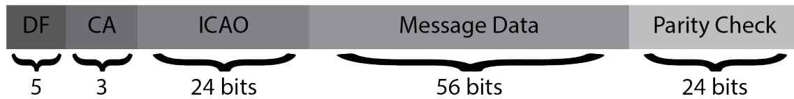
Figure 2.3: The structure of an ADS-B message.
