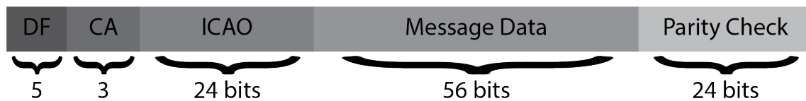
Figure 2.3: The structure of an ADS-B message.
