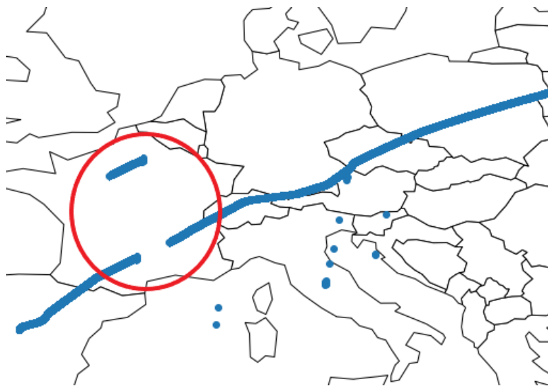
Figure 6.4: Data discrepancy from a flight between Madrid and Moscow
