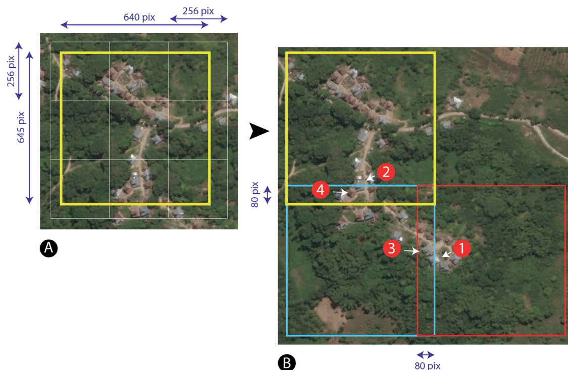
Fig. 3. Composition of images used for further deep learning. (a) images of 640 \times 645 px (in yellow) are composed by merging individual 256 \times 256 tiles (in white); (b) georeferenced images (in yellow, blue and red) overlap each other by 80 pixels in all directions; objects 1 and 2 are complete in only one image, while objects 3 and 4 are seen completely in two images. (For interpretation of the references to color in this figure legend, the reader is referred to the web version of this article.)
