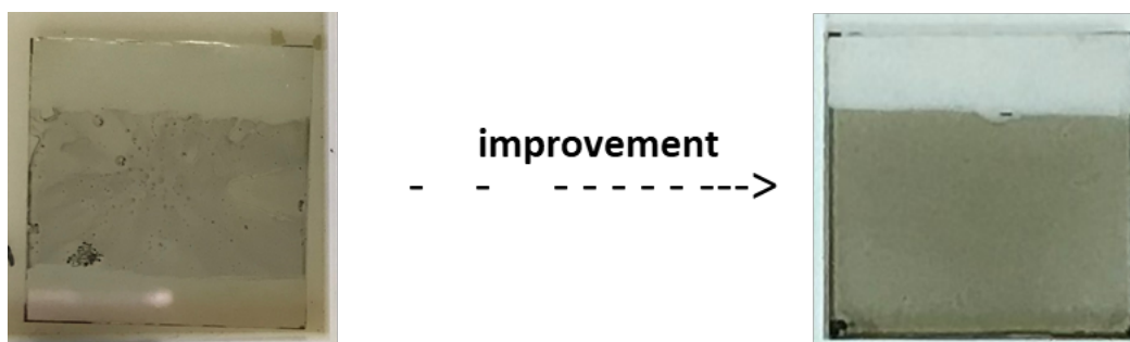
Figure 6: left: first attempts for film elaboration using spin coating, right: best homogeneous and thick film achieved after many tries – thickness of 70 nm was obtained.
