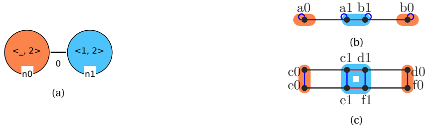
Figure 6.14: Instantiating an arc of a Jerboa graph scheme: (a) graph scheme with an arc between two nodes, (b) instantiation with the orbit graph of Figure 6.12a, and (c) instantiation with the orbit graph of Figure 6.12d.
