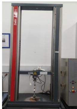
**Figure II.11: Machine de charge universelle Zwick Z005**
