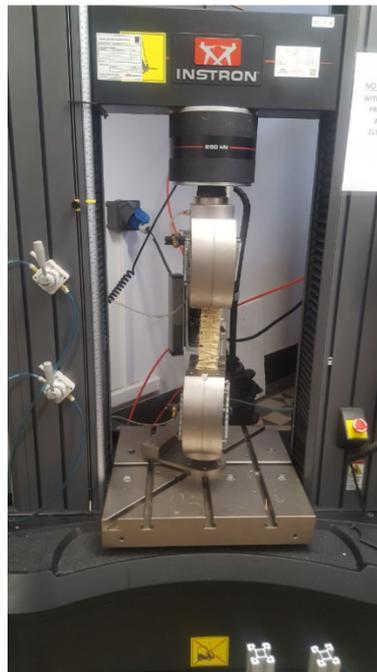
**Figure III.10: Banc de traction INSTRON 5890 250 KN**
