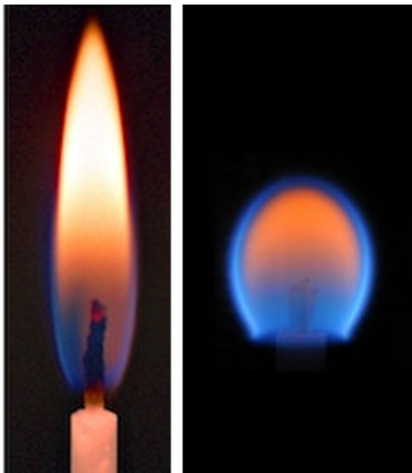
Figure 1.4: Candle flame at normal gravity in a quiescent atmosphere (left) and candle flame in microgravity with a very low velocity upward air flow (right).
