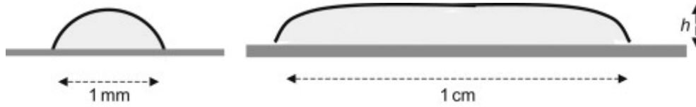
Figure 3.12: Comparison of the microdrop (left) and macrodrop (right) shapes (not at scale). Microdrops have the shape of spherical caps, whereas larger drops are flattened by the action of gravity and their height is related to the capillary length. Reproduced from Berthier (2013) [222].
