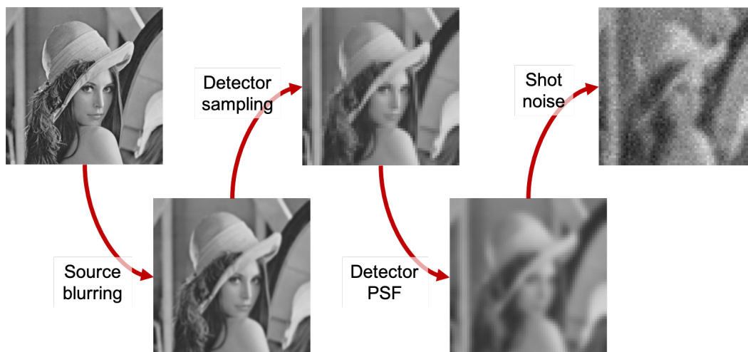
Figure 2.5: Outline of realistic image degradation for simulations: source blurring, pixel size down sampling to detector pixel size, detector PSF blurring and additional shot noise.
