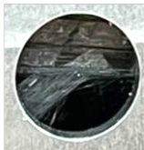
Figure 4.27: Samples used in the low energy laboratory set-up: a thin slice of a Haribo flower candy and bundles of carbon fibers.
