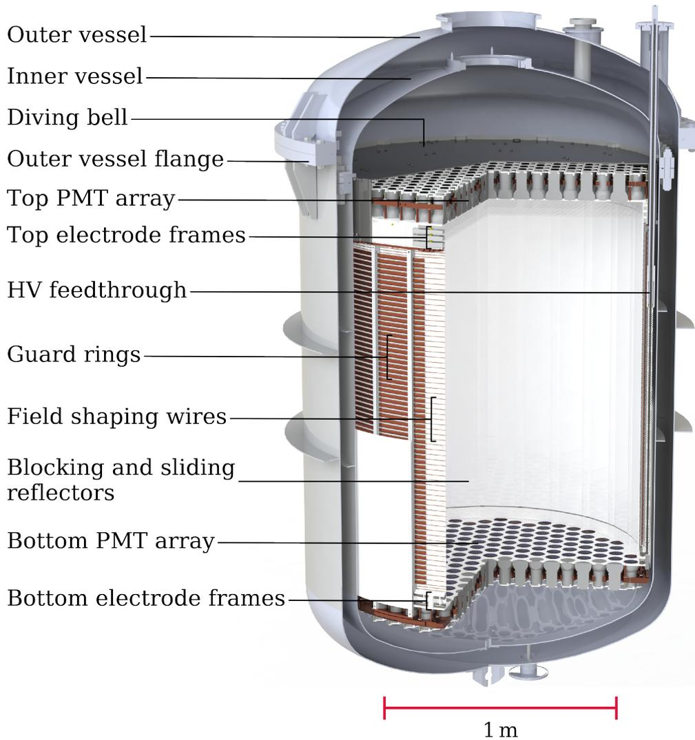
Figure 2.5: Illustration of the XENONnT cryostat and TPC
