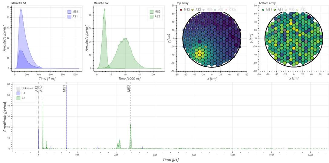
Figure 3.2: Waveform of a  $^{83m}\text{Kr}$  calibration event showing the primary S1, S2 as well as the alternate S1, S2 (see Section 2.2.10) in addition to the S2 signal tail, which corresponds to single electrons.)
