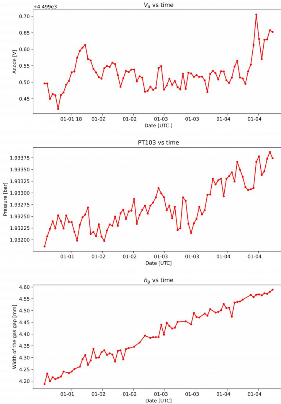
Figure 3.18: The values of the anode potential, the pressure, and the width of the gas gap corresponding to the time at which the selected data were taken (pre-SR0).
