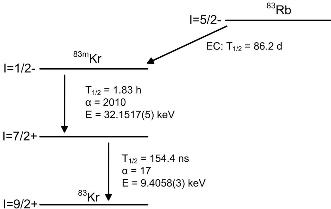
Figure 2.25: The production of the isomeric state  $^{83m}\text{Kr}$  by electron capture decay of  $^{83}\text{Rb}$ . The isomeric  $1/2^-$  state, with its half-life of 1.83 h, is populated in about 78% of all  $^{83}\text{Rb}$  decay processes and de-excites by two highly converted  $\gamma$ -transitions. Figure from [130].
