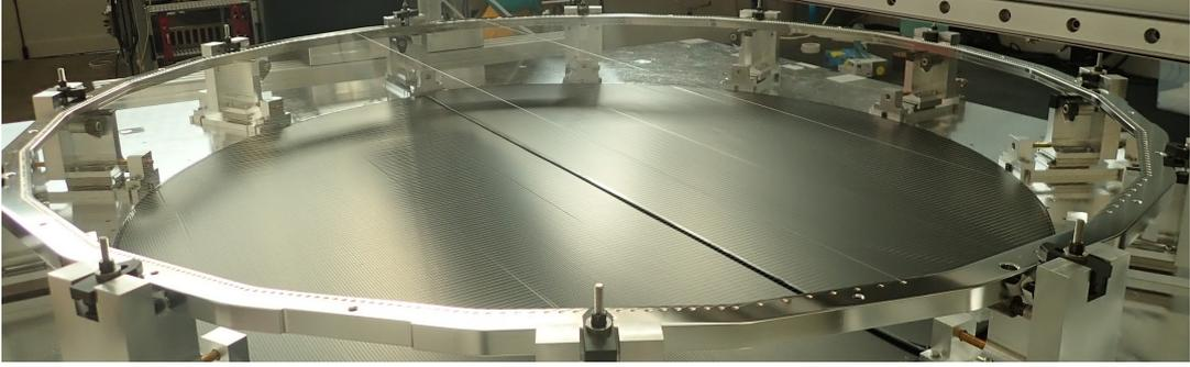
Figure 3.11: Photo of the gate where it is possible to see the two additional transverse wires.
