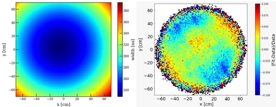
Figure 3.14: (Left) Map obtained with the fit function used. (Right) The difference between the data and the result of the fit function for each bin. The fact that the fit is not centered in  $(x, y)$  suggests that the TPC is not perfectly vertical, and this translation of the center is therefore related to gravitational effects.
