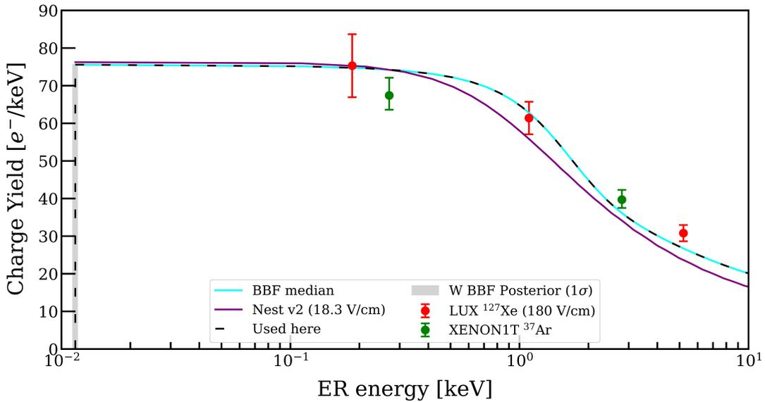
Figure 2.28: The results on the charge yield for the  $^{37}\text{Ar}$  L peak and K peak energies (green dots) obtained from XENON1T data are compared with other measurements of the charge yield at different energies. The cyan line is the prediction from BBF, and the violet line is the prediction from NEST. The dotted vertical bar represents the value of 11.5 eV, which is the work function value of the Xenon used.
