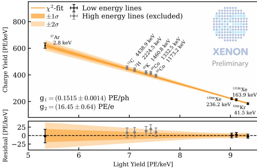
Figure 2.4: Calculation of  $g_1$  and  $g_2$  in XENONnT. This was performed using multiple mono-energetic lines with known energies to extract the best fit for the value of the gains ( $g_1, g_2$ ) by making a “Doke plot”, a plot in charge yield and light yield space. Different energy or different electric field are expected to have different charge yield and light yield, but these points will only move along the line as the total quanta number is fixed.
