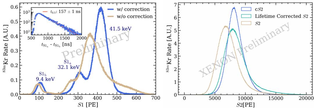
Figure 2.22: (Left)  $^{83m}\text{Kr}$  S1 spectra before and after S1 (x,y,z) correction under 18 V/cm drift field. The S1 resolution is much better after correction. Inset plot: The time difference between  $^{83m}\text{Kr}$  double scatters. The fitted  $157 \pm 1$  ns half-life is close to the literature value of 156 ns. (Right) Distributions of S2, electron lifetime corrected S2 and cS2 under 18.3 V/cm drifting field.
