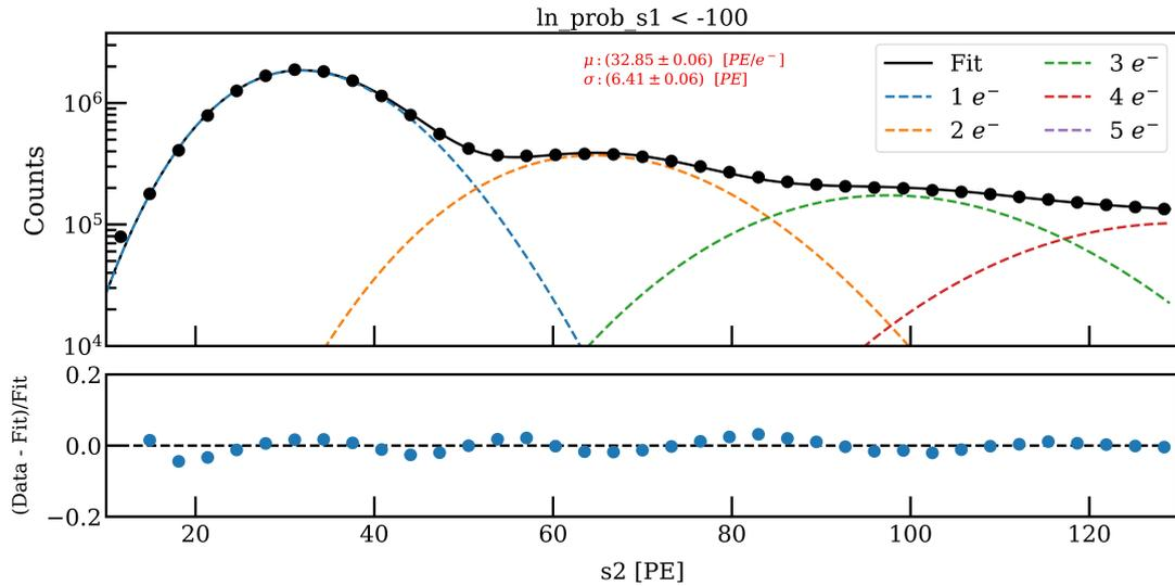
Figure 3.7: The fit plot of the SE spectrum with model (3.4), choosing  $N = 5$ . In this figure, it is possible to see the value given by the fit for the secondary scintillation gain  $\mu$ , its standard deviation  $\sigma$ , and the contribution of each electron population to the spectrum. The value  $\ln\_prob\_s1 < -100$  indicates the probability limit chosen to cut the S1 (see Section 2.2.9).
