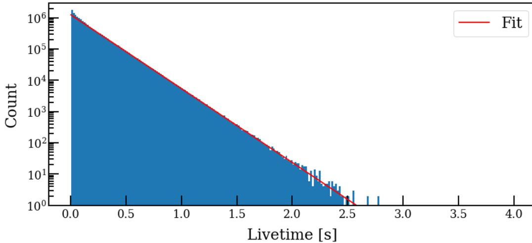
Figure 3.40: Primary S2 live-time distribution. In red the fit of the distribution with a power law.
