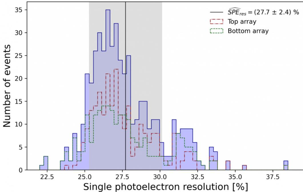
Figure 2.10: SPE resolution defined as  $\sigma_{1PE}/\mu_{1PE}$  for the two PMT arrays (top and bottom) + total. The mean and the standard deviation come from the fitting of the SPE spectrum, with very low illumination LED data calibration. The solid black line shows the average SPE resolution.
