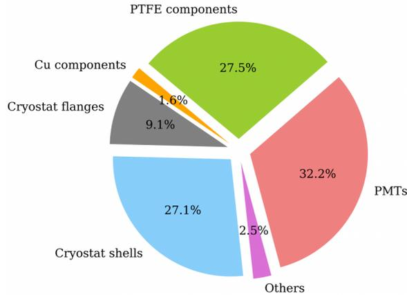
Figure 2.32: Main NR background source by material component.
