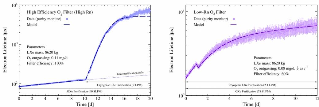
Figure 2.14: (Left) Electron lifetime improvement after the start of cryogenic LXe purification with the high-efficiency  $O_2$  filter. (Right) Electron lifetime improvement after switching to cryogenic LXe purification with the low-Rn  $O_2$  filter.
