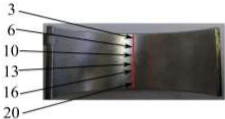
Figure 3.22 Roughness Measurement locations
