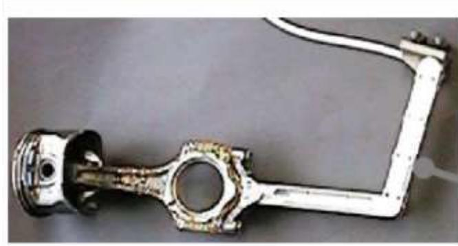
Figure 1.17 Merritt connecting rod grass hopper linkage [26]
