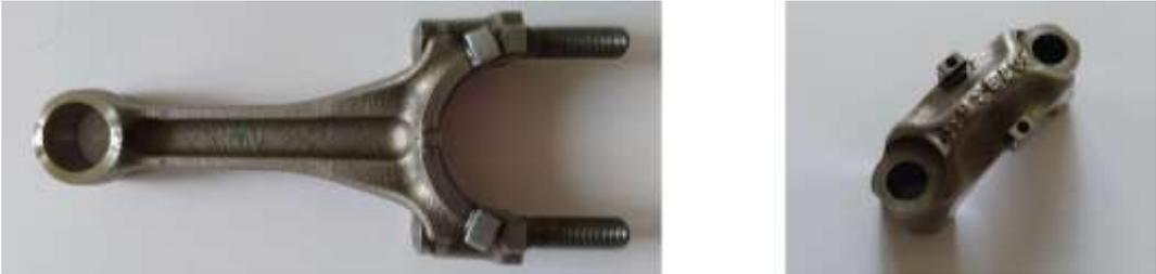
Figure 2.27 Eddy current gap sensors mounts
