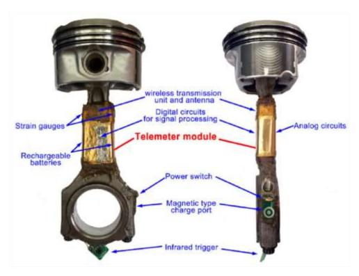
Figure 1.18 Fang telemetry system on a connecting rod [17], [28]
