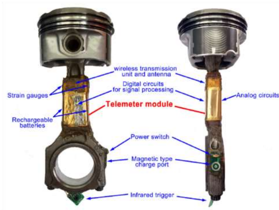
Figure 1.18 Fang telemetry system on a connecting rod [17], [28]
