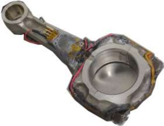
Figure A.7 The connecting rod after curing the Araldite® 2014-2 glue
