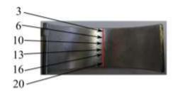
Figure 3.22 Roughness Measurement locations
