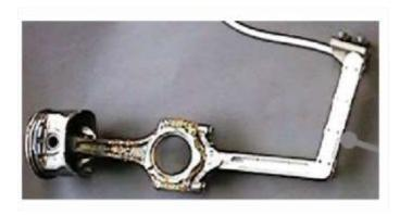
Figure 1.17 Merrit connecting rod grass hopper linkage [26]
