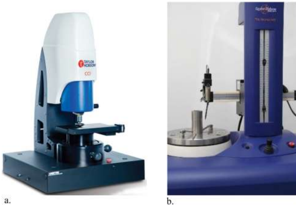
Figure 2.12 Surface topology measurement machines: a.: Talysurf CCI 6000; b. Talysond 356
