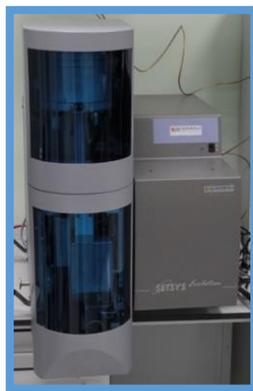
Figure 41: SETSYS evolution equipment Setaram TGA equipment
