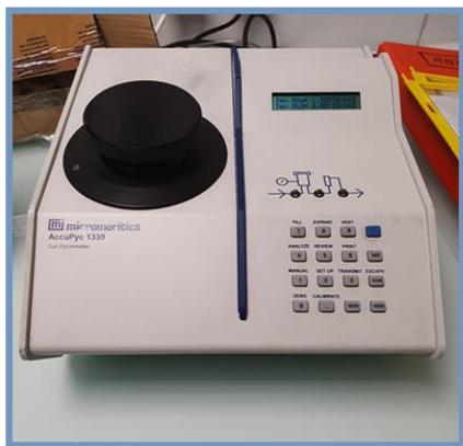
Figure 52: Ac-cuPyc 1330 (Micrometrics) helium pycnometer
