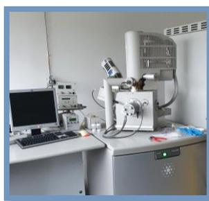
Figure 39: SEM FEI Quanta 200 FEG (Fisher Thermo Scientific) machine
