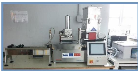
Figure 62: Process 11 twin-screw extruder
