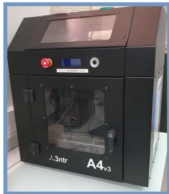
Figure 51: A4v3 FFF 3D printer
