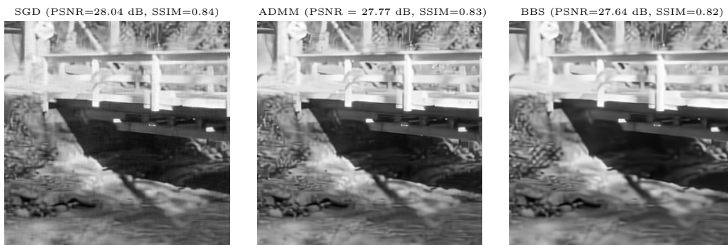
Figure 4.7: Plug & Play deblurring, for a 9 \times 9 kernel, an additive Gaussian noise of standard deviation \sigma^2 = (1/255)^2 , for \varepsilon = (5/255)^2 and for the nearly optimal value of \alpha = 0.3 .
