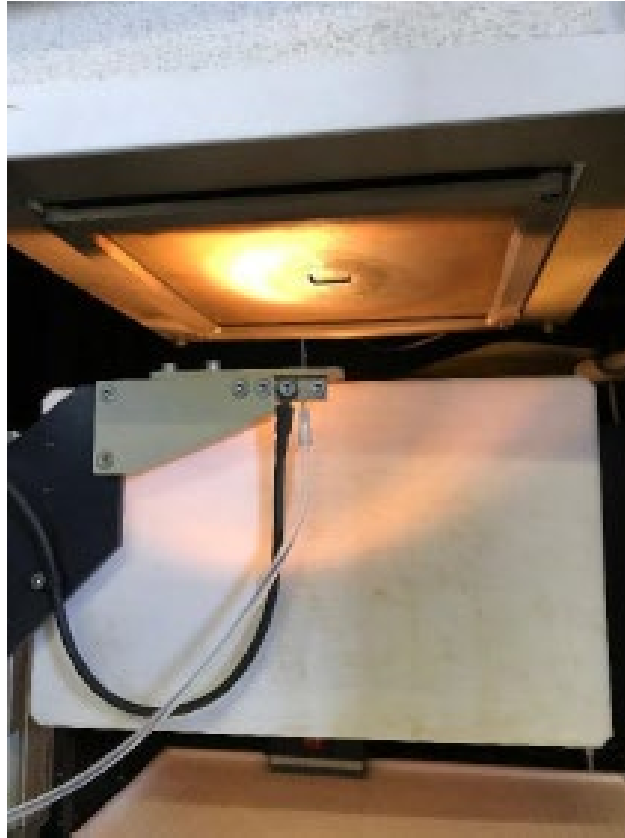
Figure 4.1 Picture of electrostatic spray deposition setup
