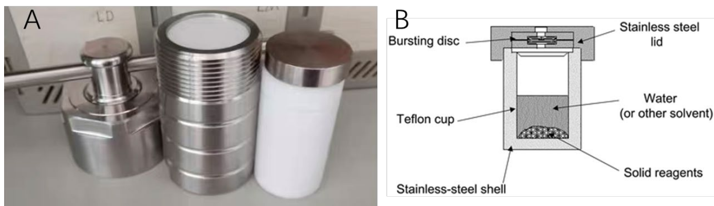
Figure 5.7 A) Photograph of the used autoclave; B) schematic of a Teflon TM -lined, stainless-steel autoclave typically used in the laboratory to perform solvothermal synthesis. Adapted from Ref 10 10 .
